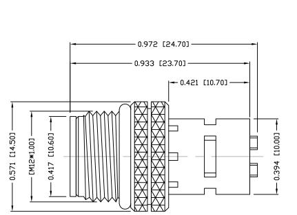
NΠΤΕ: MATERIAL HOUSING: PBT UL94V-0, BLACK CONTACT: BRASS NUT: BRASS □-RING: EPDM, BLACK SHELL: BRASS FINISH CONTACT: GOLD PLATED □VER 504" NICKEL NUT: NICKEL PLATED SHELL: BRIGHT TIN PLATED ELECTRICAL RATED CURRENT: 4A RATED VOLTAGE: 60V INSULATION RESISTANCE: 100 MOhms MIN. CONTACT RESISTANCE: 10 mOhms MAX. IP67 WATER PROOF: **ENVIRONMENT** -40°C TD +85°C OPERATION TEMPERATURE: MAX WIRE AWG: 22
