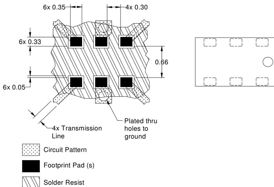
Dimensions are in Millimeters
