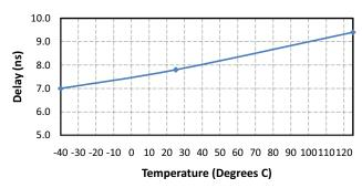
Figure 15. Propagation Delay vs. Temperature
