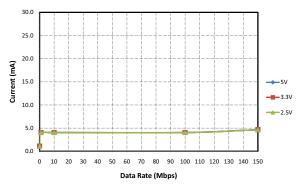
Figure 9. Si8650/55 Typical V<sub>DD1</sub> Supply Current vs. Data Rate 5, 3.3, and 2.5 V Operation
