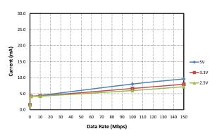
Figure 10. Si8651 Typical V<sub>DD1</sub> Supply Current vs. Data Rate 5, 3.3, and 2.5 V Operation (15 pF Load)
