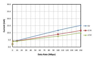
Figure 11. Si8652 Typical V<sub>DD1</sub> Supply Current vs. Data Rate 5, 3.3, and 2.5 V Operation (15 pF Load)
