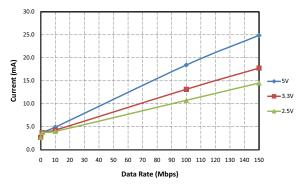
Figure 13. Si8651 Typical V<sub>DD2</sub> Supply Current vs. Data Rate 5, 3.3, and 2.5 V Operation (15 pF Load)
