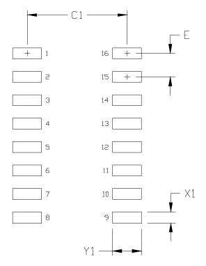
Figure 19. 16-Pin Narrow Body SOIC PCB Land Pattern
