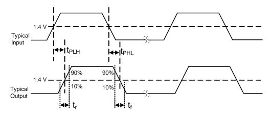
Figure 2. Propagation Delay Timing
