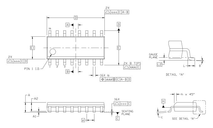
Figure 18. 16-pin Small Outline Integrated Circuit (SOIC) Package
