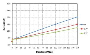
Figure 14. Si8652 Typical V<sub>DD2</sub> Supply Current vs. Data Rate 5, 3.3, and 2.5 V Operation (15 pF Load)
