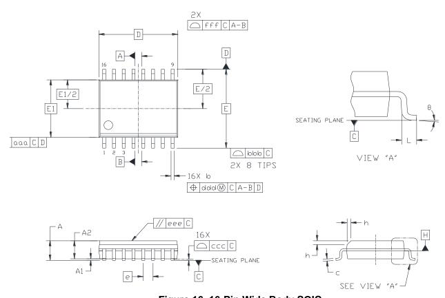
Figure 16. 16-Pin Wide Body SOIC
