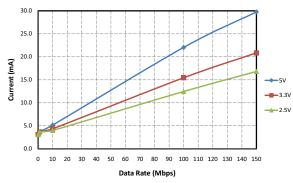
Figure 12. Si8650/55 Typical V<sub>DD2</sub> Supply Current vs. Data Rate 5, 3.3, and 2.5 V Operation (15 pF Load)
