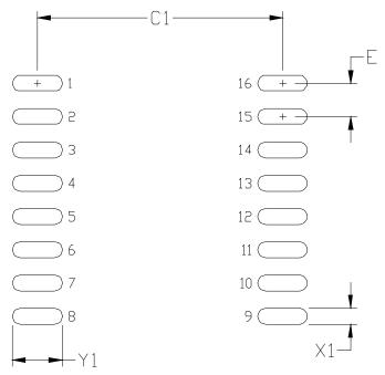
Figure 17. 16-Pin SOIC Land Pattern
