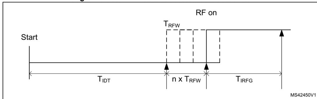
Figure 19. Direct command NFC Response Field ON
