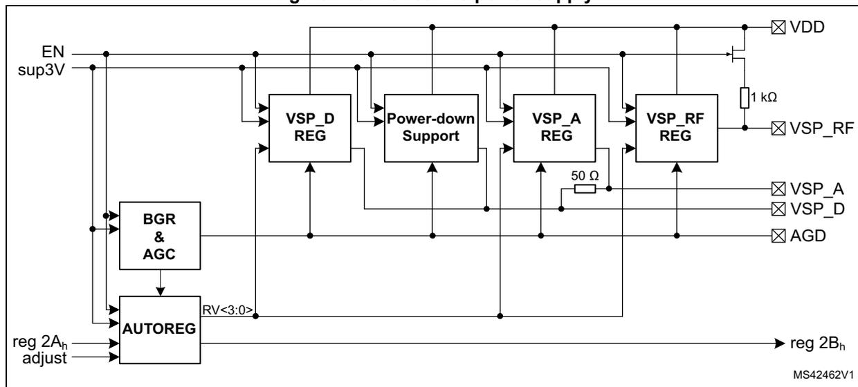
Figure 7 shows the building blocks of the ST25R3912/3 power supply system and the signals that control it.
