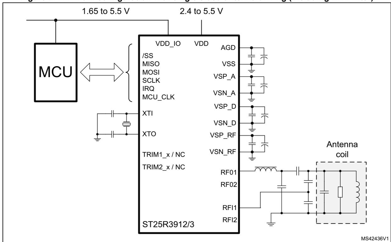
Figure 3. Minimum configuration with differential antenna driving (including EMC filter)
