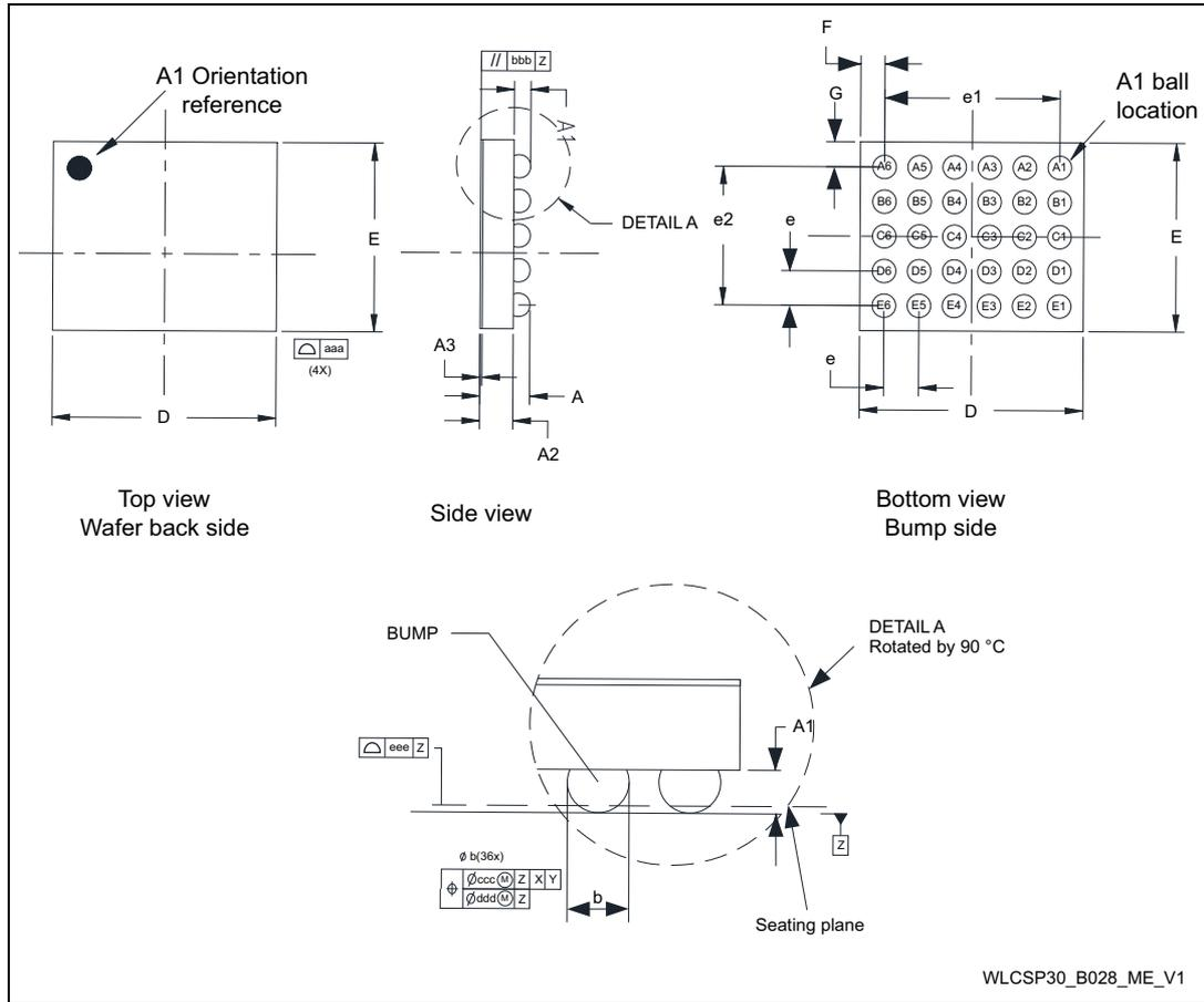
Table 104. WLCSP30 30-ball, 3.065 x 2.865 mm, 0.5 mm pitch wafer level chip scale mechanical data
