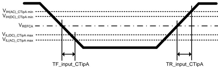
**Figure 156. CS# and Input A Slew Rate Definition**
