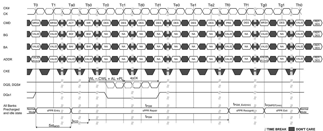
Figure 161. Fail Row Soft PPR (WR Case)
