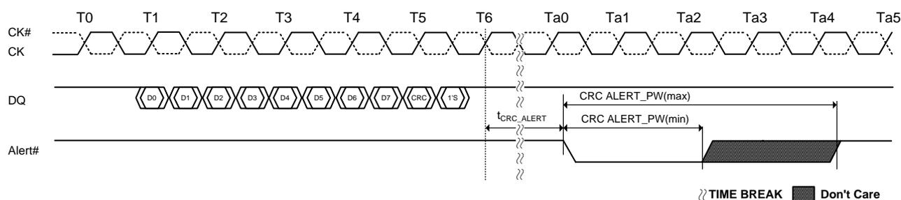
NOTE 1. CRC ALERT\_PW IS Specified from the point Where the DRAM starts to drive the signal low to the point where the DRAM driver releases and the controller starts to pull the signal up.
