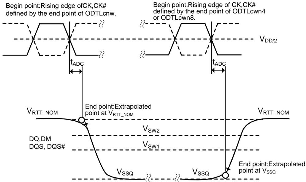
**Figure 175. Definition of  $t_{ADC}$  at Dynamic ODT Control**
