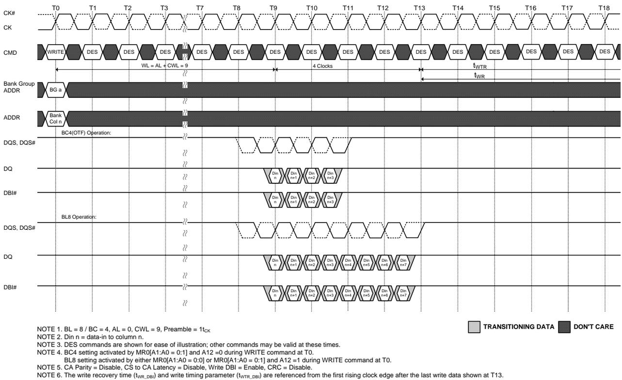
**Figure 146. WRITE (BL8/BC4) OTF with  $1t_{CK}$  Preamble and DBI**
