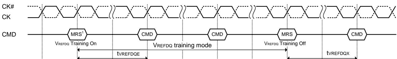
NOTE 1. The MR command used to enter  $V_{REFDQ}$  Calibration Mode treats MR6 A [5:0] as don’t care while the next subsequent MR command sets  $V_{REFDQ}$  values in MR6 A[5:0].
