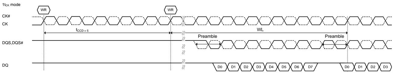
2tCK mode:  $t_{CCD}=5$  is not allowed in 2tCK mode
