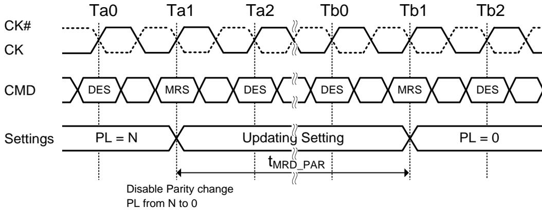
NOTE 1.  $t_{MRD\_PAR} = t_{MOD} + N$ ; where N is the programmed parity latency prior to the MRS command exiting CA parity mode.
