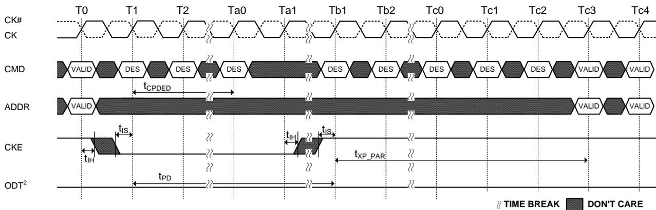
NOTE 1 VALID command at T0 is ACT, DES or Precharge with still one bank remaining open after completion of the precharge command.
