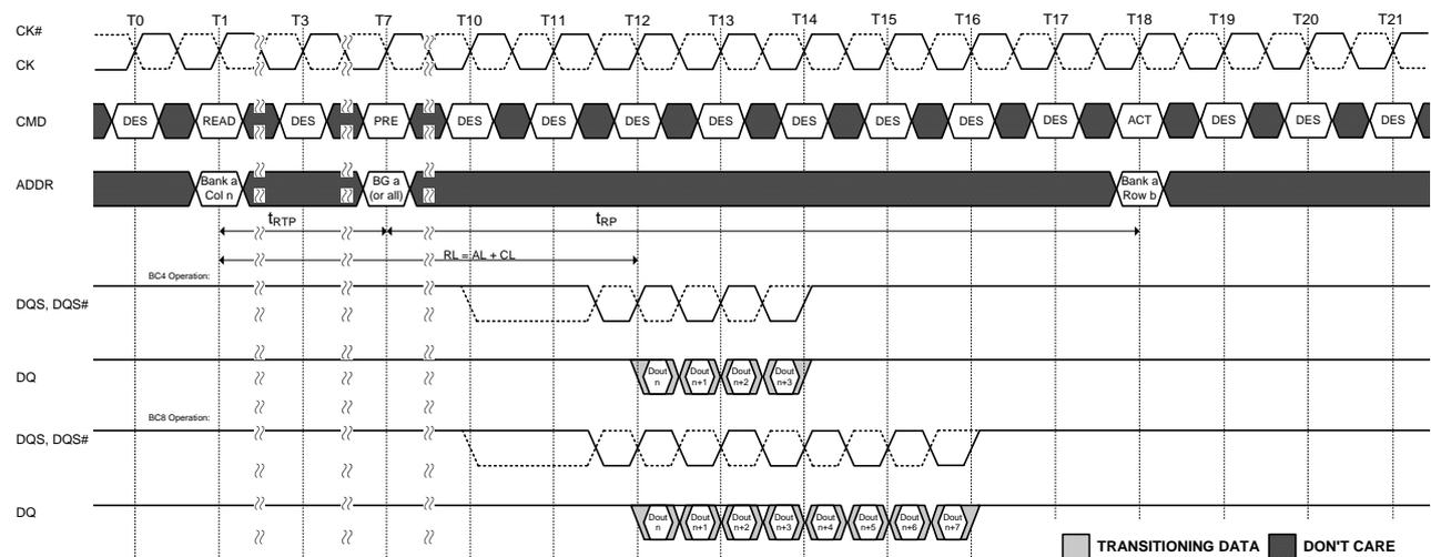
NOTE 1. BL = 8, RL = 11 (CL = 11, AL = 0), Preamble =  $2t_{CK}$ ,  $t_{RTP} = 6$ ,  $t_{RP} = 11$
