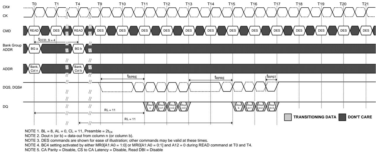
**Figure 96. READ (BC4) to READ (BC4) with 2t<sub>CK</sub> Preamble in Different Bank Group**
