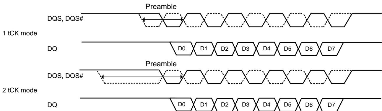
**Figure 78. 1 $t_{CK}$  vs. 2 $t_{CK}$  WRITE Preamble Mode**
