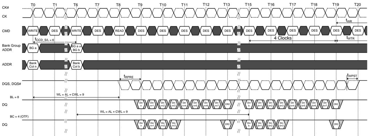
NOTE 1. BL = 8, AL = 0, CWL = 9, Preamble =  $1t_{CK}$ ,  $t_{CCD\_SIL} = 6$
