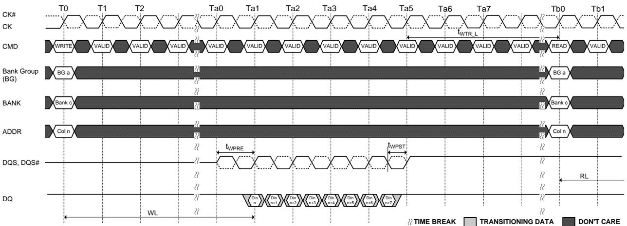
**Figure 77. t<sub>WTR\_L</sub> Timing (WRITE to READ, Same Bank Group, CRC and DM Disabled)**
