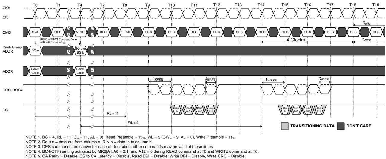
**Figure 105. READ (BC4) to READ (BL8) OTF with 1t<sub>CK</sub> Preamble in Different Bank Group**
