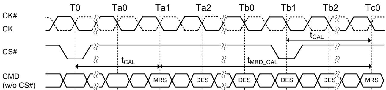
NOTE1: MRS at Ta1 may or may not modify CAL,  $t_{MRD\_CAL}$  is computed based on new  $t_{CAL}$  setting.
