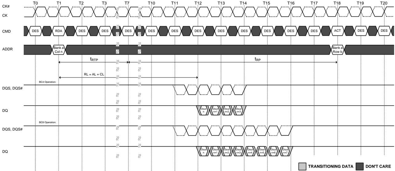
NOTE 1. BL = 8, RL = 11 (CL = 11, AL = 0), Preamble = 1t<sub>CK</sub>, t<sub>RTP</sub> = 6, t<sub>RP</sub> = 11
