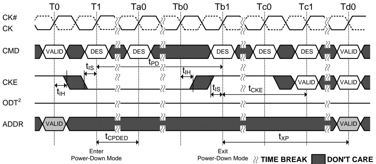
NOTE 1. Valid command at T0 is ACT, DES or Precharge with still one bank remaining open after completion of the precharge command.
