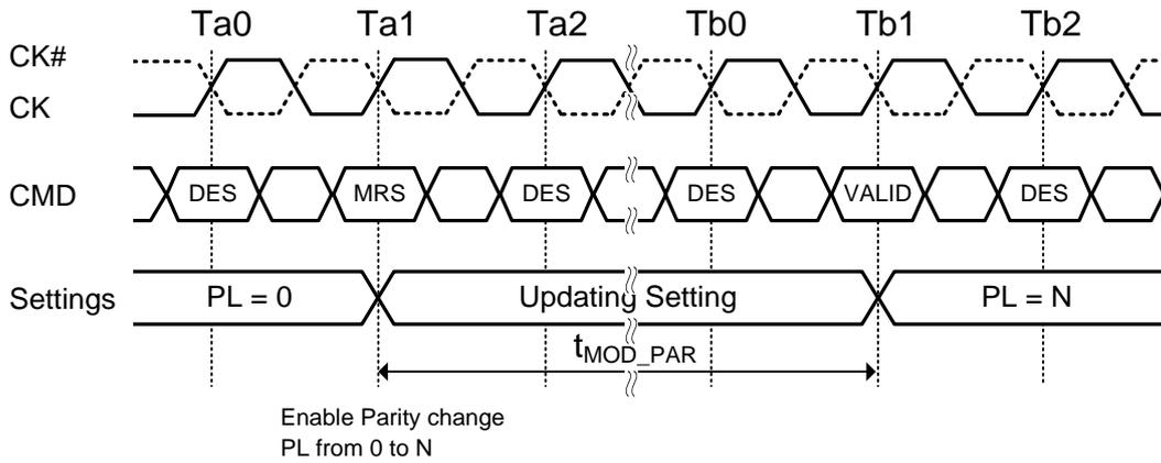
NOTE 1.  $t_{MOD\_PAR} = t_{MOD} + N$ ; where N is the programmed parity latency with the MRS command entering CA parity mode.
