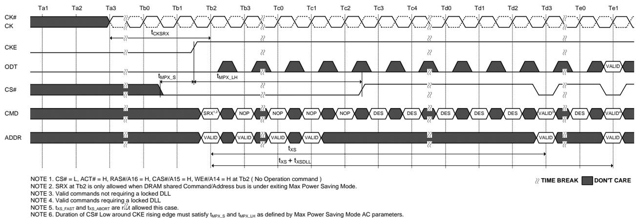
Figure 26. Self Refresh Exit with No Operation command
