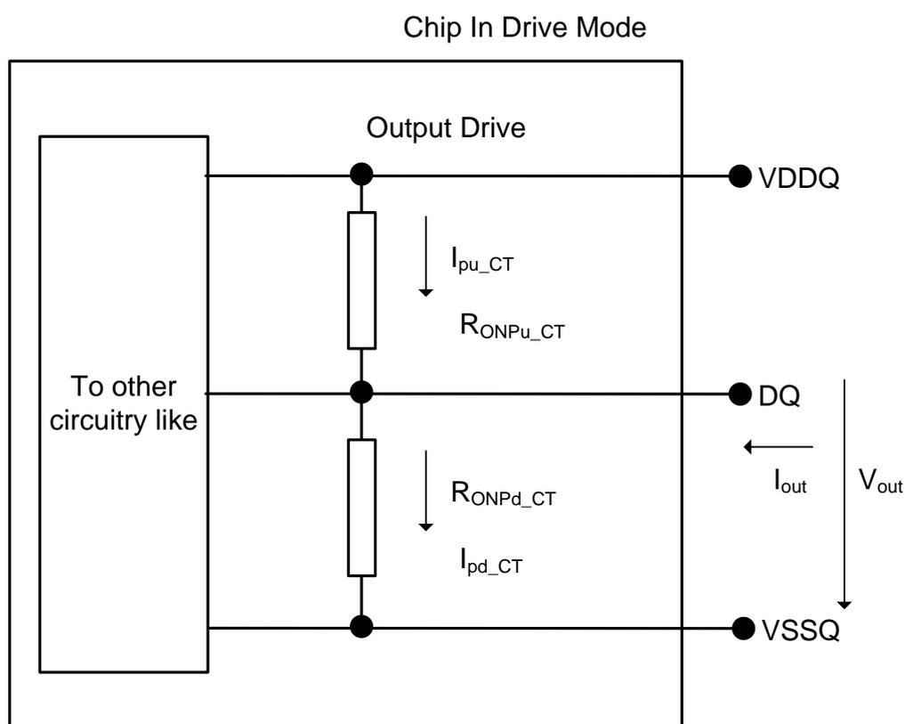
Figure 181. Output Driver Characteristic of Connectivity Test
