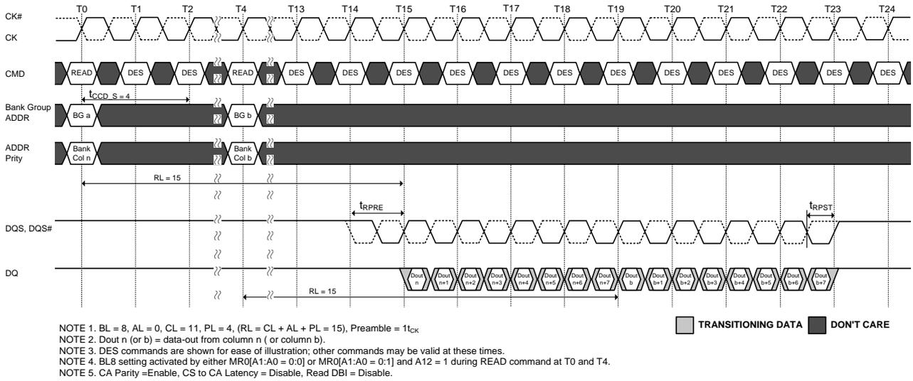
Figure 117. Consecutive READ (BL8) with 1t<sub>CK</sub> Preamble and CA Parity in Different Bank Group
