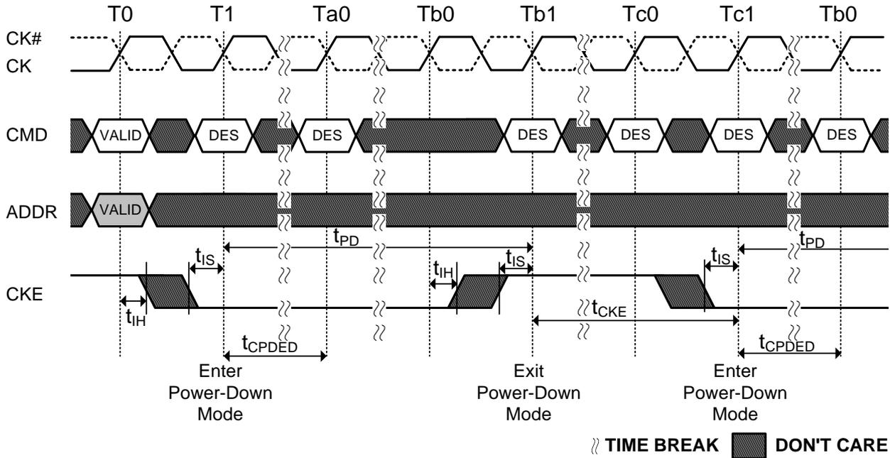
Figure 37. Power-Down Entry/Exit Clarification
