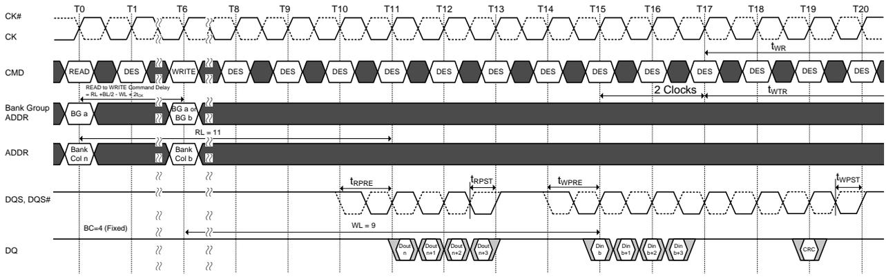
NOTE 1. BC = 4 (Fixed), RL = 11 (CL = 11, AL = 0), Read Preamble = 1t<sub>CK</sub>, WL=9 (CWL=9, AL=0), Write Preamble = 1t<sub>CK</sub>
