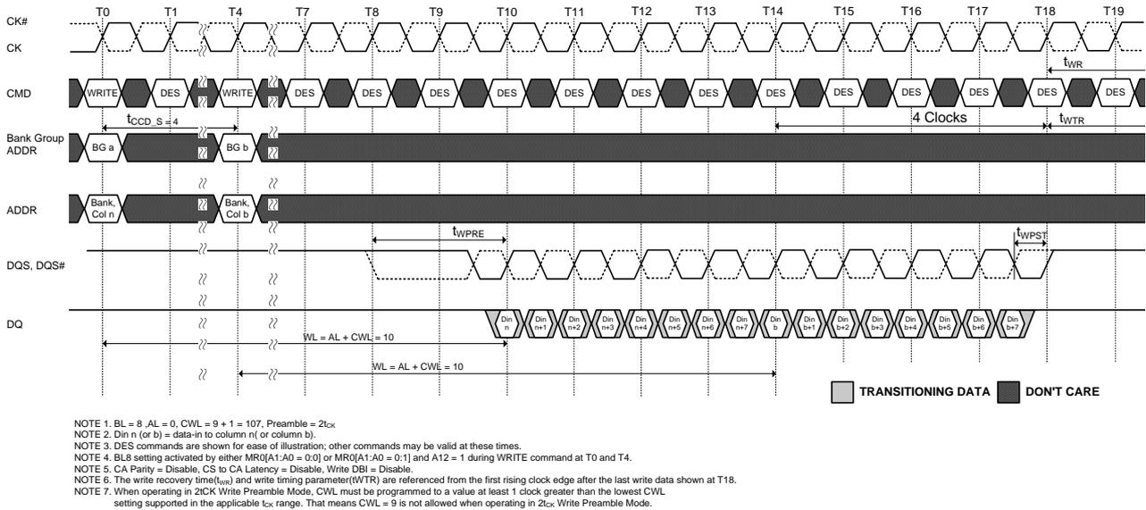
**Figure 128. Consecutive WRITE (BL8) with 2t<sub>CK</sub> Preamble in Different Bank Group**
