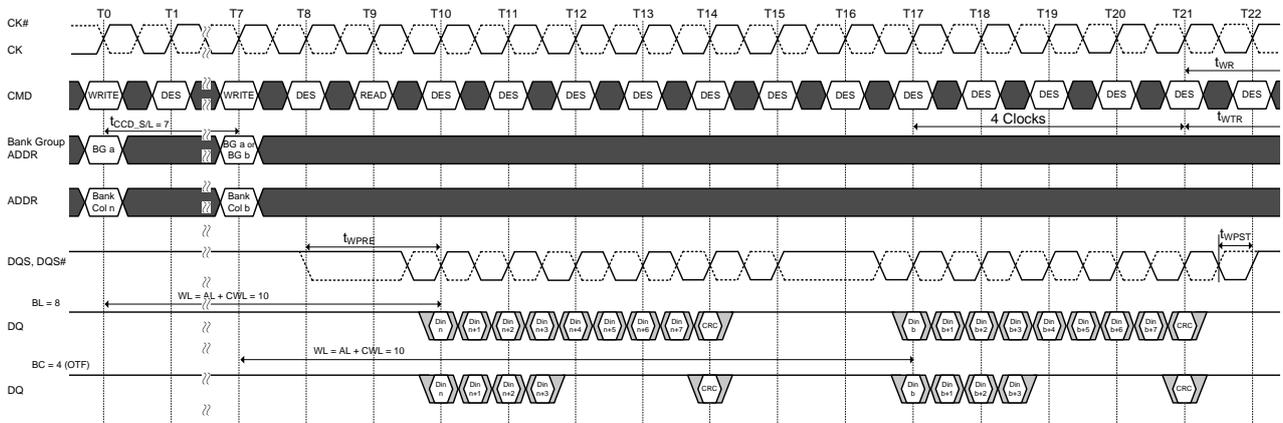
NOTE 1. BL = 8, AL = 0, CWL =  $9 + 1 = 10$ , Preamble =  $2t_{CK}$ ,  $t_{CCD\_SIL} = 7$
