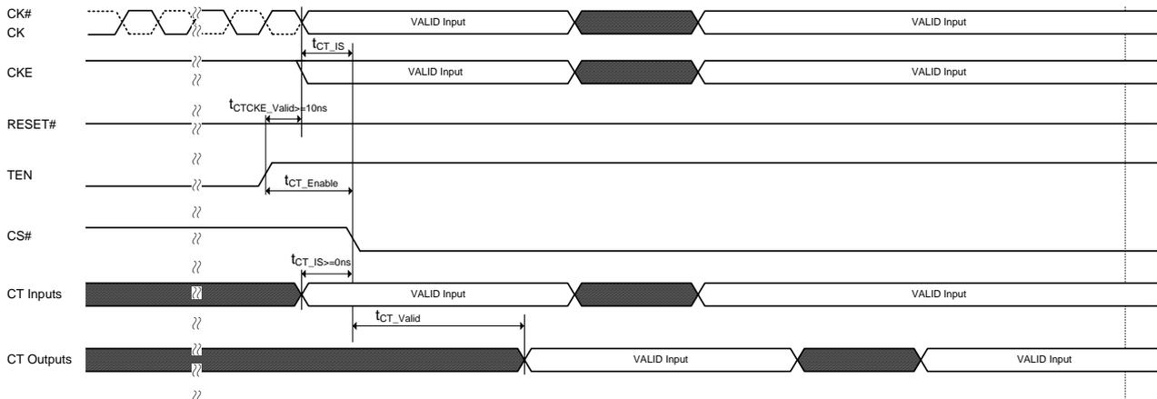
Figure 154. Timing Diagram for Connectivity Test(CT) Mode
