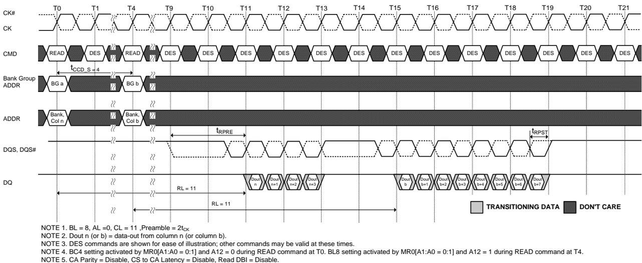
**Figure 106. READ (BC4) to READ (BL8) OTF with 2t<sub>CK</sub> Preamble in Different Bank Group**
