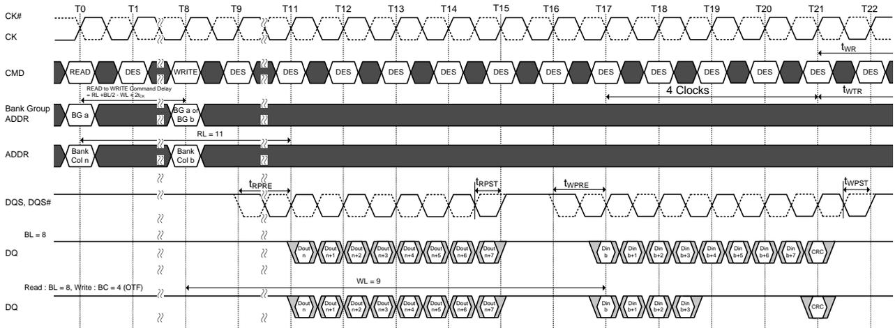
NOTE 1. BL = 8 ( or BC = 4 : OTF for Write), RL = 11 (CL = 11, AL = 0), Read Preamble = 1t<sub>CK</sub>, WL=9 (CWL=9, AL=0), Write Preamble = 1t<sub>CK</sub>
