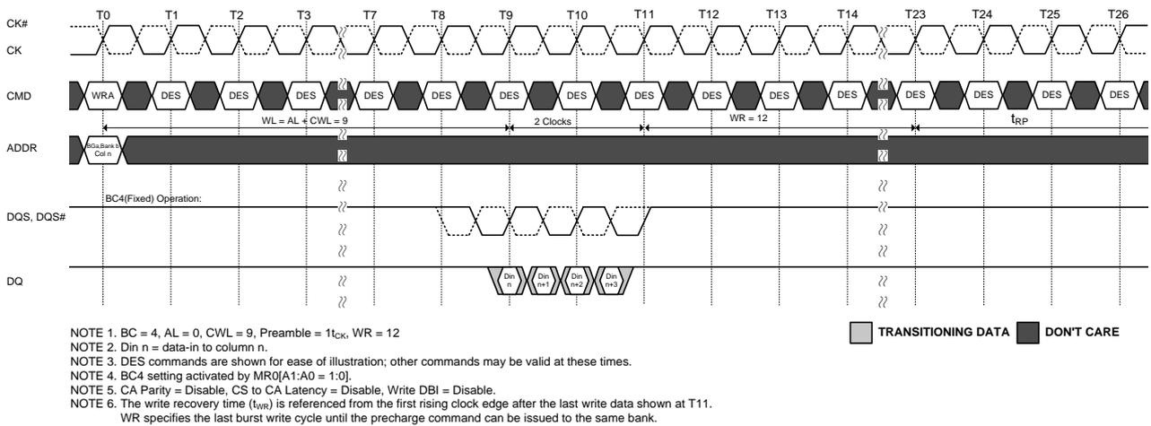
**Figure 145. WRITE (BC4) Fixed with Auto PRECHARGE Operation and  $1t_{CK}$  Preamble**
