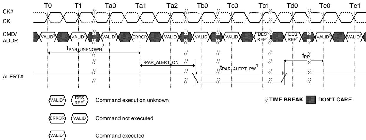
NOTE 1. DRAM is emptying queues, Precharge All and parity checking off until Parity Error Status bit cleared.
