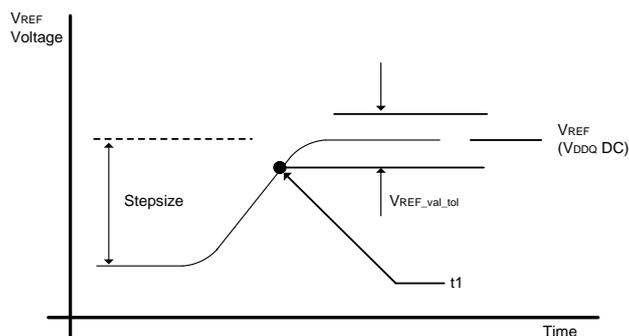
**Figure 48. V<sub>REF</sub> step single stepsize increment case**
