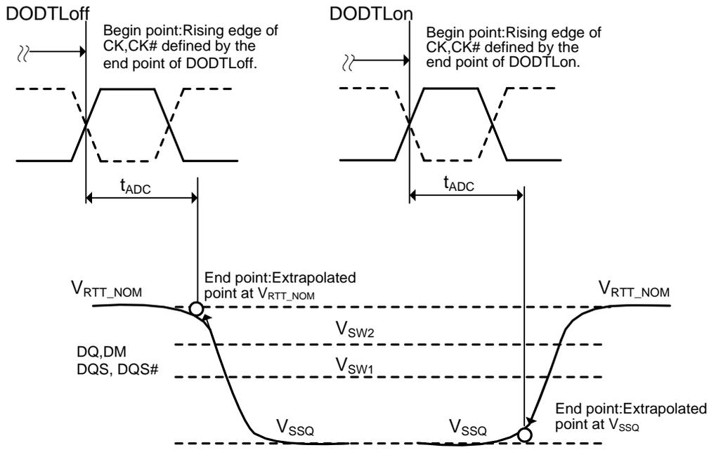
**Figure 174. Definition of  $t_{ADC}$  at Direct ODT Control**
