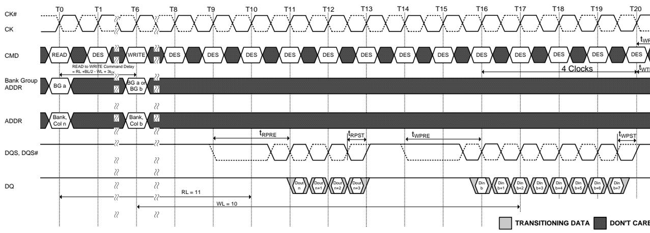
NOTE 1. BC = 4, RL = 11 (CL = 11, AL = 0), Read Preamble =  $2t_{CK}$ , WL = 10 (CWL = 9 +  $1^{10}$ , AL = 0), Write Preamble =  $2t_{CK}$
