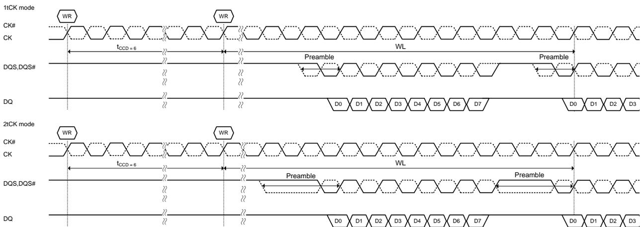
**Figure 81.  $t_{CCD}=6$  (AL=PL=0)**
