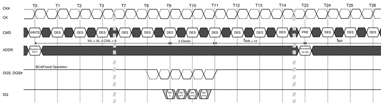
NOTE 1. BC = 4, AL = 0, CWL = 9, Preamble =  $1t_{CK}$ ,  $t_{WR} = 12$
