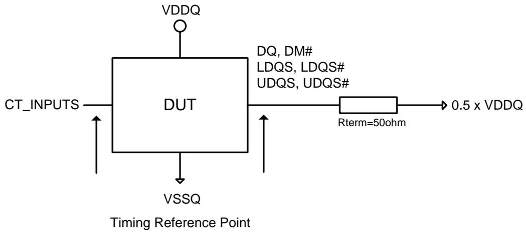
**Figure 182. Connectivity Test Mode Timing Reference Load**
