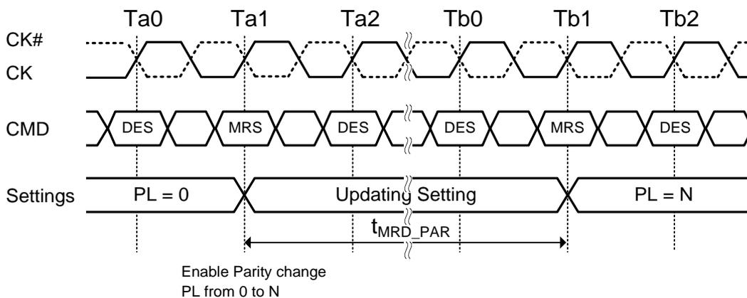
NOTE 1.  $t_{MRD\_PAR} = t_{MOD} + N$ ; where N is the programmed parity latency with the MRS command entering CA parity mode.
