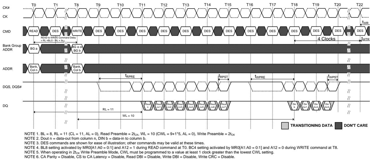
**Figure 110. READ (BL8) to WRITE (BC4) OTF with 2t<sub>CK</sub> Preamble in Same or Different Bank Group**
