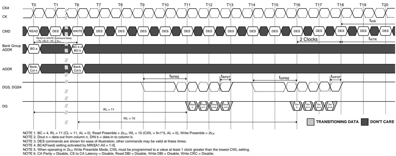
**Figure 102. READ (BC4) Fixed to WRITE (BC4) Fixed with  $2t_{CK}$  Preamble in Same or Different Bank Group**
