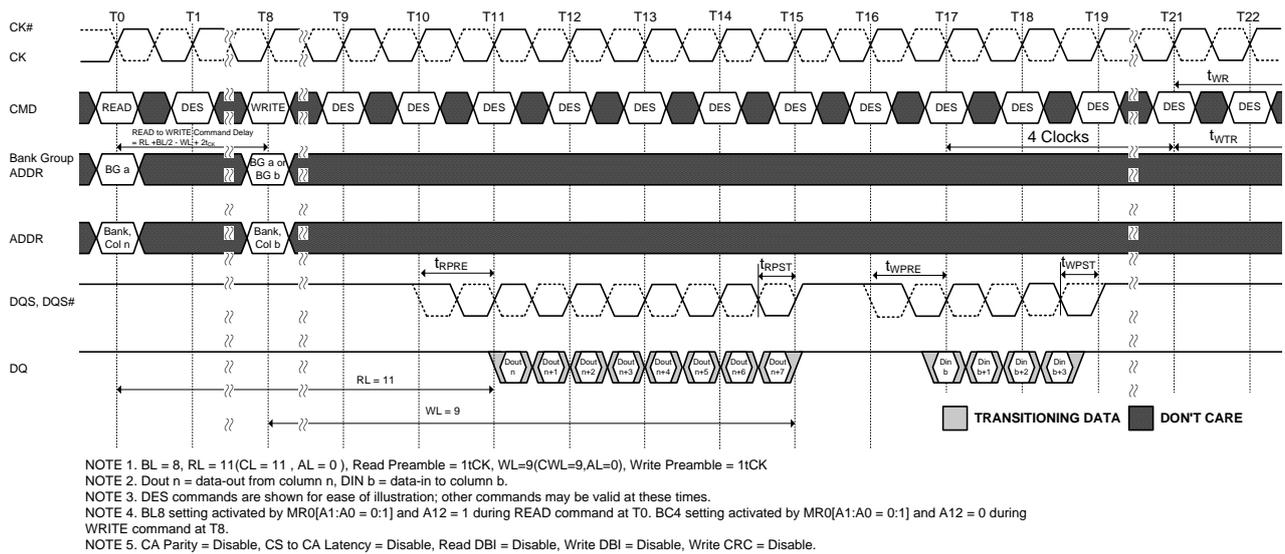
**Figure 109. READ (BL8) to WRITE (BC4) OTF with 1t<sub>CK</sub> Preamble in Same or Different Bank Group**
