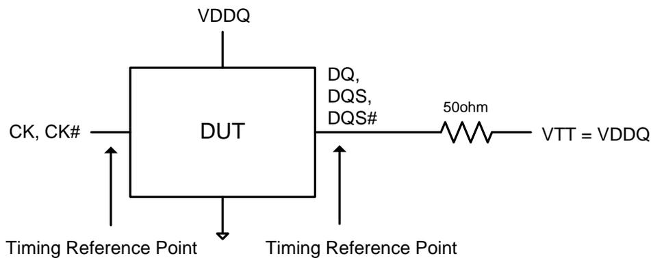
**Figure 183. Reference Load for AC Timing and Output Slew Rate**
