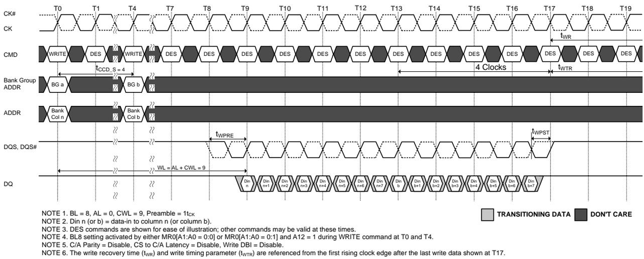
**Figure 127. Consecutive WRITE (BL8) with 1t<sub>CK</sub> Preamble in Different Bank Group**
