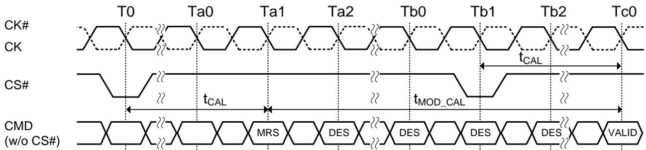
NOTE1: MRS at Ta1 may or may not modify CAL,  $t_{MOD\_CAL}$  is computed based on new  $t_{CAL}$  setting.
