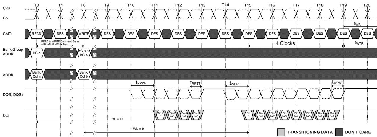
NOTE 1. BC = 4, RL = 11 (CL = 11, AL = 0), Read Preamble =  $1t_{CK}$ , WL = 9 (CWL = 9, AL = 0), Write Preamble =  $1t_{CK}$
