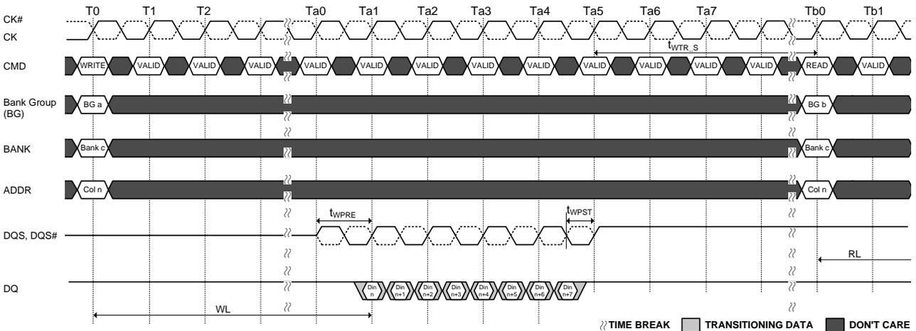
**Figure 76. t<sub>WTR\_S</sub> Timing (WRITE to READ, Different Bank Group, CRC and DM Disabled)**
