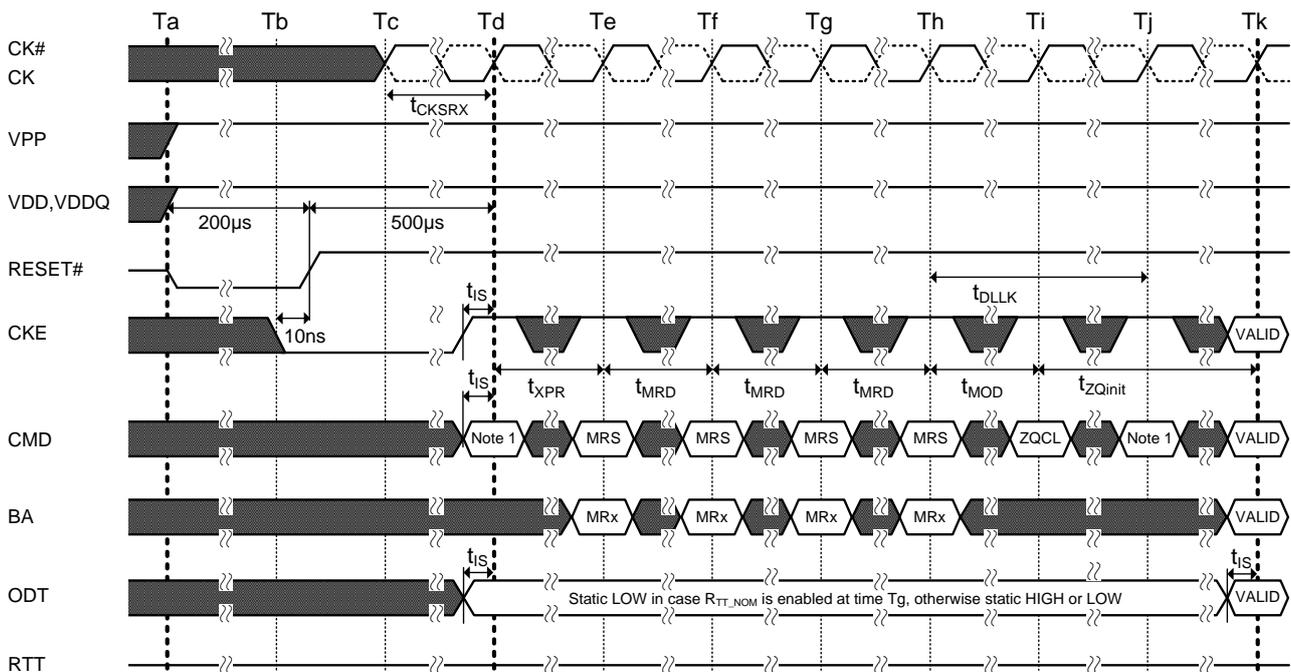
NOTE 1. From time point "Td" until "Tk" DES commands must be applied between MRS and ZQCL commands.
