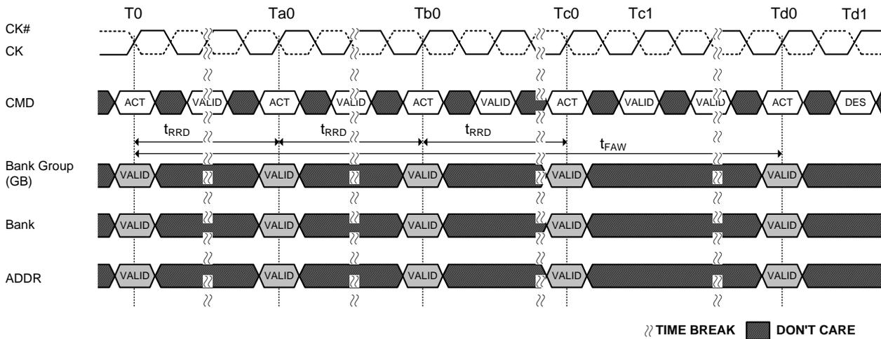
**Figure 75. t<sub>FAW</sub> Timing**
