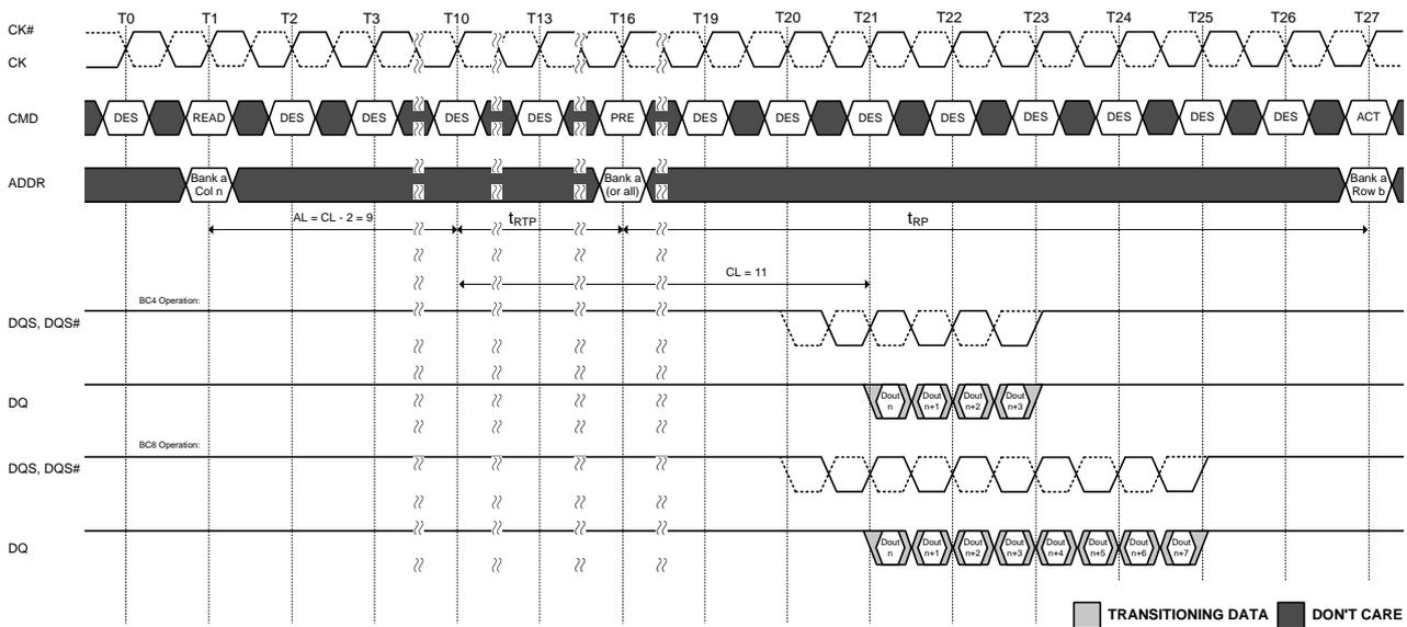
NOTE 1. BL = 8, RL = 20 (CL = 11, AL = CL - 2), Preamble = 1t<sub>CK</sub>, t<sub>RTP</sub> = 6, t<sub>RP</sub> = 11
