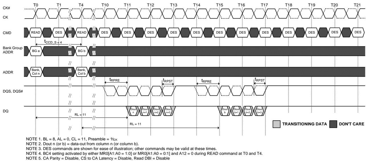
**Figure 95. READ (BC4) to READ (BC4) with 1t<sub>CK</sub> Preamble in Different Bank Group**
