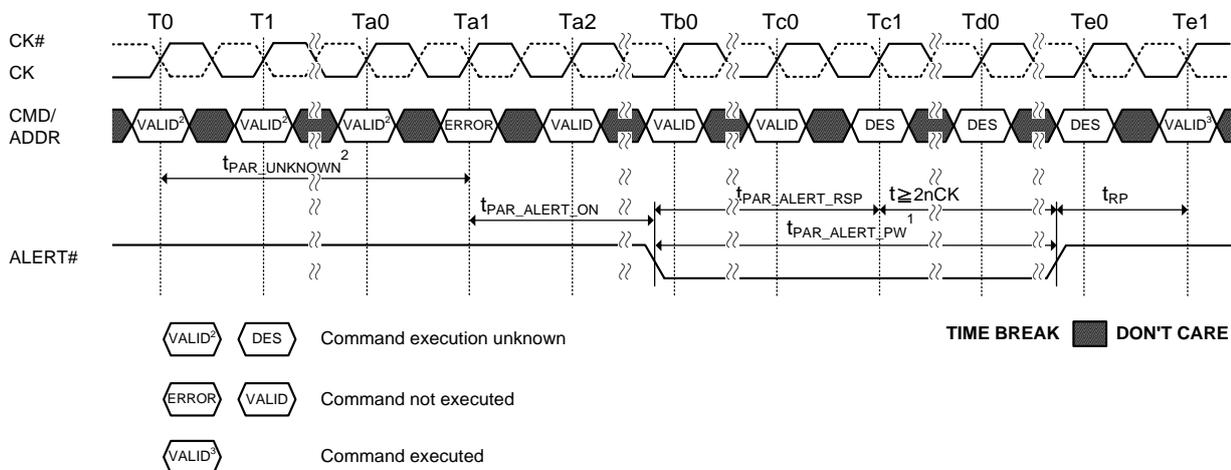
NOTE 1. DRAM is emptying queues, Precharge All and parity check re-enable finished by tPAR\_ALERT\_PW.
