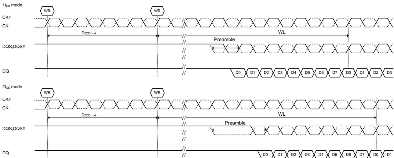
**Figure 79.  $t_{CCD}=4$  (AL=PL=0)**
