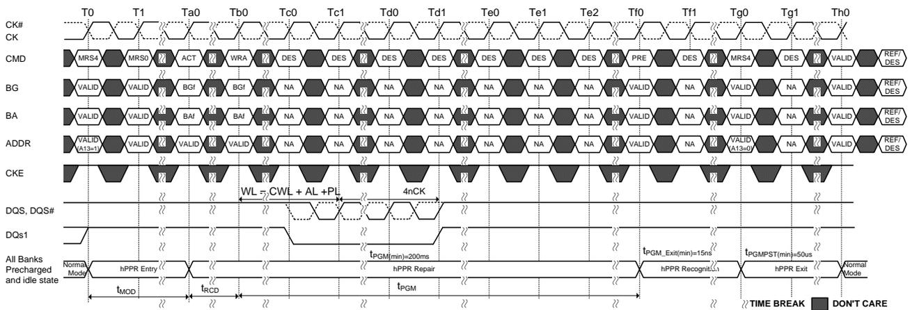
**Figure 160. Hard Fail Row Repair (WR Case)**
