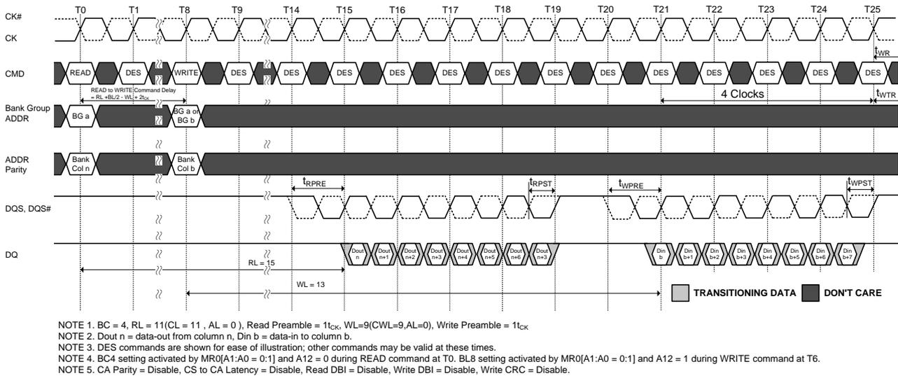
Figure 118. READ (BL8) to WRITE (BL8) with 1t<sub>CK</sub> Preamble and CA parity in Same or Different Bank Group
