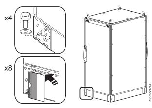
3. Connect the cabinet frame to the Building Common Bonding Network (grounding equipment not provided).
