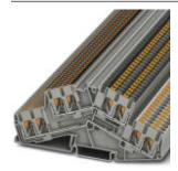
Double-level terminal block, With equipotential bonder, Cross section: 0.14 mm<sup>2</sup> - 4 mm<sup>2</sup>, AWG: 26 - 12, Connection type: Push-in connection, Width: 5.2 mm, Color: gray, Mounting type: NS 35/7,5, NS 35/15
