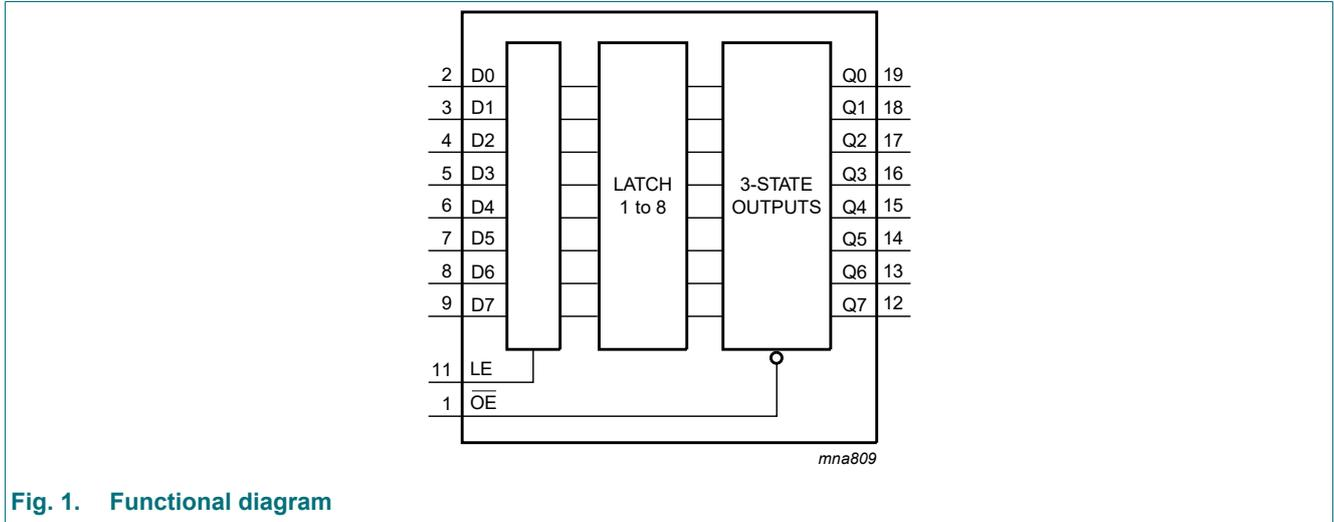
Fig. 1. Functional diagram
