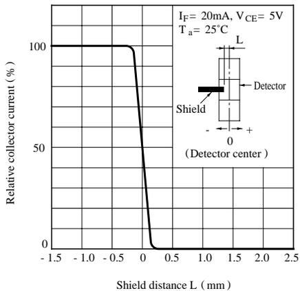
**Fig.13 Relative Collector Current vs. Shield Distance (2)**
