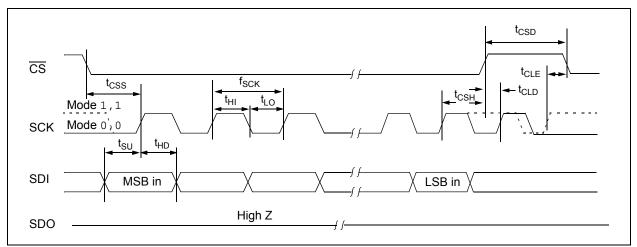
FIGURE 1-2: Serial Input Timing Diagram.
