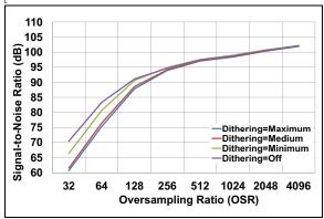
FIGURE 2-13: SNR vs.OSR.
