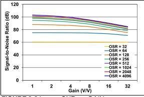
**FIGURE 2-21:** SNR vs. GAIN.
