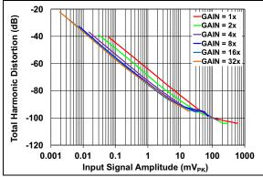
**FIGURE 2-23:** THD vs. Input Signal Amplitude.
