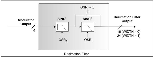
FIGURE 5-3: MCP3910 Decimation Filter Block Diagram.
