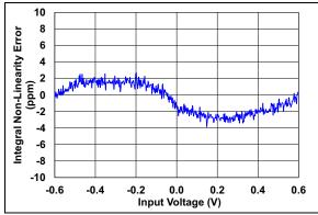
FIGURE 2-35: Integral Non-Linearity (Dithering Maximum).
