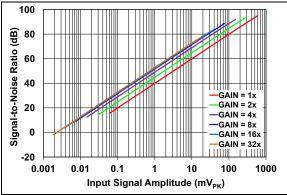
FIGURE 2-25: SNR vs. Input Signal Amplitude.
