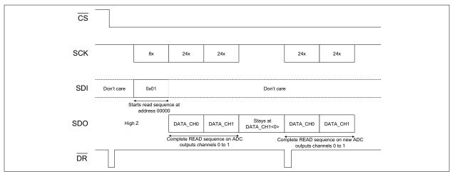
FIGURE 6-7: Typical Continuous Read Communication (WIDTH\_DATA<1:0> = 01, SPI Mode 0,0).
