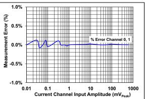
**FIGURE 2-6:** Measurement Error with 2-Point Calibration.
