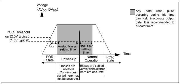
FIGURE 5-8: Power-On Reset Operation.
