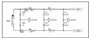
**FIGURE 8-7:** Second-Order Anti-Aliasing Filter for Rogowski Coil-Based Designs.
