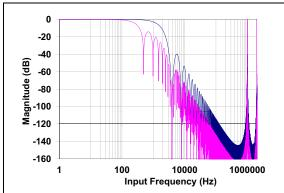
FIGURE 5-5: SINC Filter Frequency
