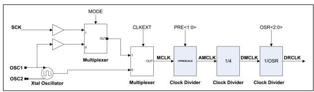
FIGURE 4-1: Clock Sub-Circuitry.
