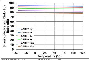
FIGURE 2-29: SINAD vs. Temperature.
