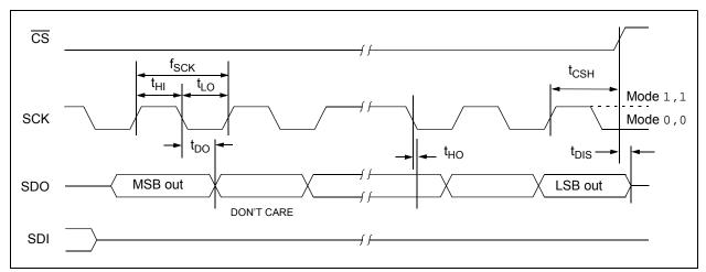
FIGURE 1-1: Serial Output Timing Diagram.
