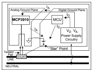
FIGURE 8-5: Connection Diagram.
