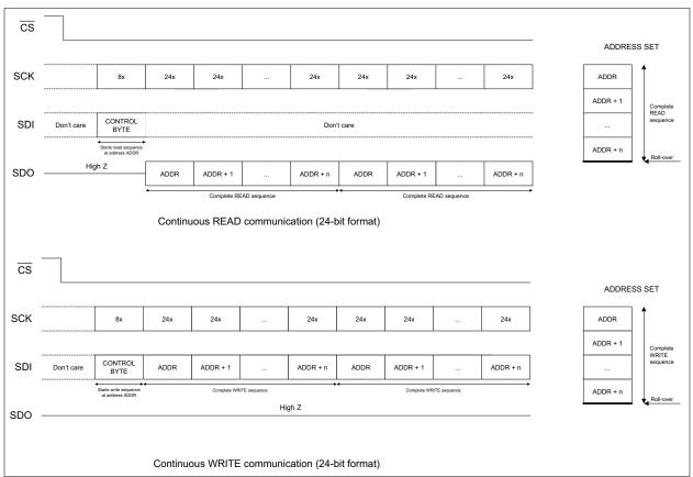
FIGURE 6-6: Continuous Communication Sequences.
