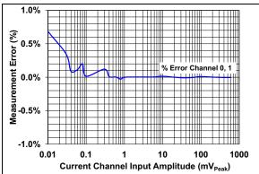
FIGURE 2-5: Measurement Error with 1-Point Calibration.
