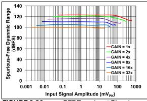
FIGURE 2-26: SFDR vs. Input Signal Amplitude.
