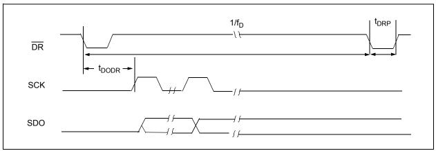
FIGURE 1-3: Data Ready Pulse/Sampling Timing Diagram.
