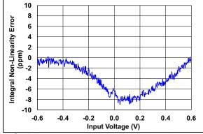
FIGURE 2-36: Integral Non-Linearity (Dithering Off).
