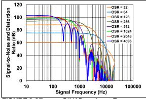
FIGURE 2-27: SINAD vs. Input Frequency.
