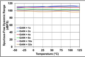
FIGURE 2-31: SFDR vs. Temperature.
