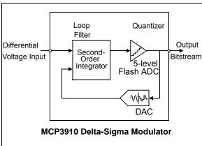
FIGURE 5-1: Simplified Delta-Sigma ADC Block Diagram.
