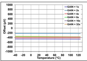
FIGURE 2-32: Offset vs. Temperature vs. Gain.
