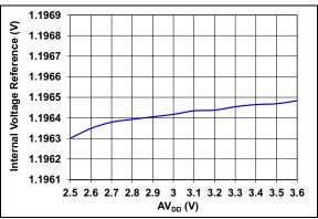
**FIGURE 2-34:** Internal Voltage Reference vs. Supply Voltage.
