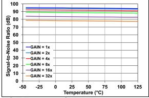
FIGURE 2-30: SNR vs. Temperature.
