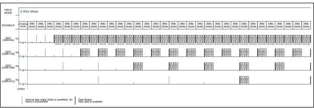
FIGURE 7-3: MCP3910 2-Wire Communication Protocol.
