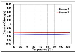
**FIGURE 2-33:** Channel Offset Matching vs. Temperature.
