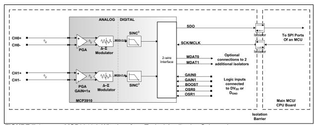
FIGURE 7-1: MCP3910 2-Wire Interface Typical Application Schematic.
