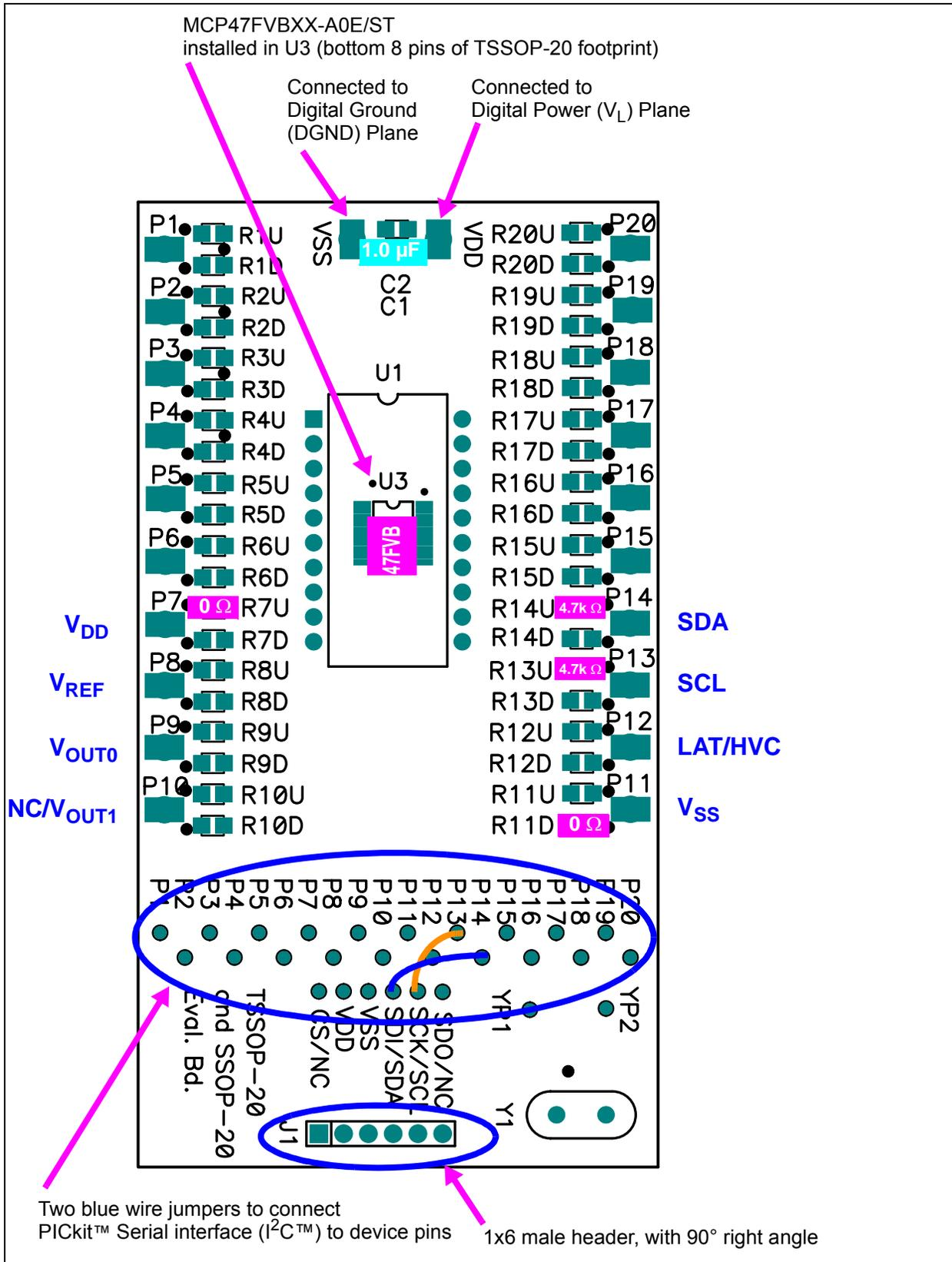
**FIGURE 9-1:** MCP47FVBXX Evaluation Board Circuit Using TSSOP20EV.
