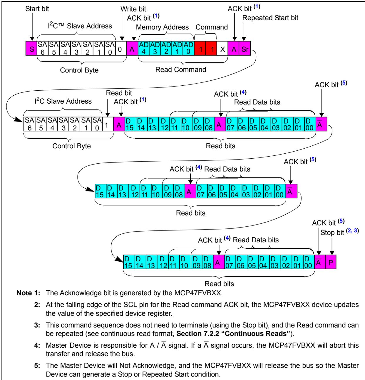
**FIGURE 7-7:** Continuous Read Command Of Specified Address.
