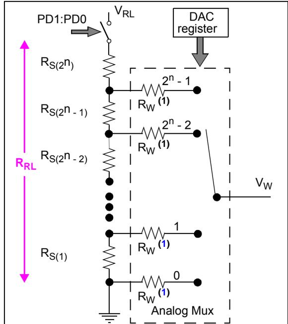
$$V_W = \frac{\text{DAC Register Value}}{\# \text{ Resistor in Resistor Ladder}} \times V_{RL}$$
