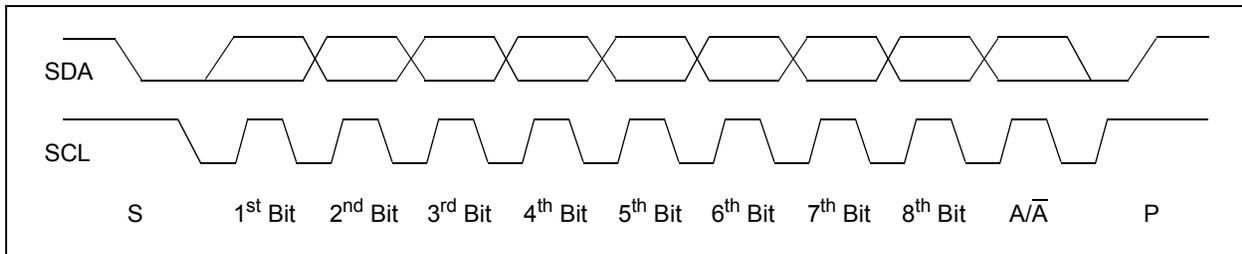
**FIGURE B-7:** Typical 8-Bit I<sup>2</sup>C Waveform Format.
