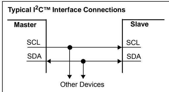
FIGURE B-1: Typical I<sup>2</sup>C Interface.
