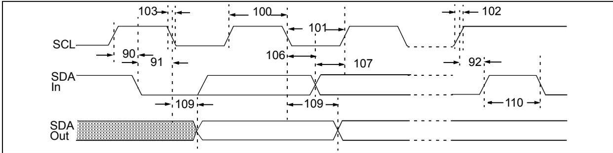
**FIGURE 1-6:** I<sup>2</sup>C™ Bus Timing Waveforms.
