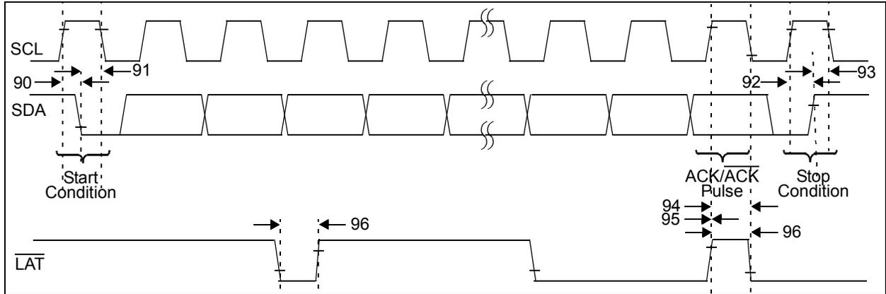
**FIGURE 1-4:**  $I^2C^{TM}$  Bus Start/Stop Bits Timing Waveforms.
