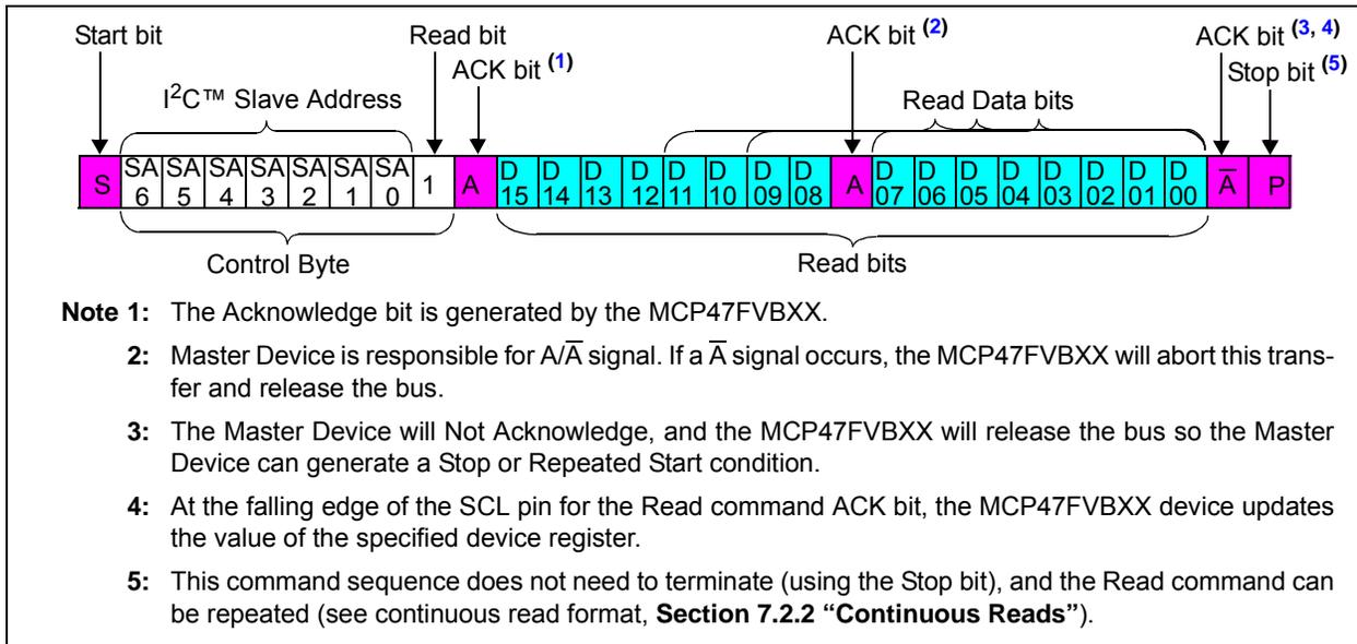
**FIGURE 7-5:** Read Command - Last Memory Address Accessed.
