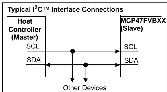
FIGURE 6-1: Typical I<sup>2</sup>C Interface.
