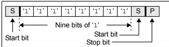
**FIGURE 8-9:** Software Reset Sequence Format.
