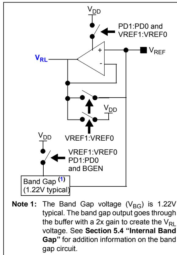
**Note 1:** The Band Gap voltage ( $V_{BG}$ ) is 1.22V typical. The band gap output goes through the buffer with a 2x gain to create the  $V_{RL}$  voltage. See Section 5.4 "Internal Band Gap" for addition information on the band gap circuit.
