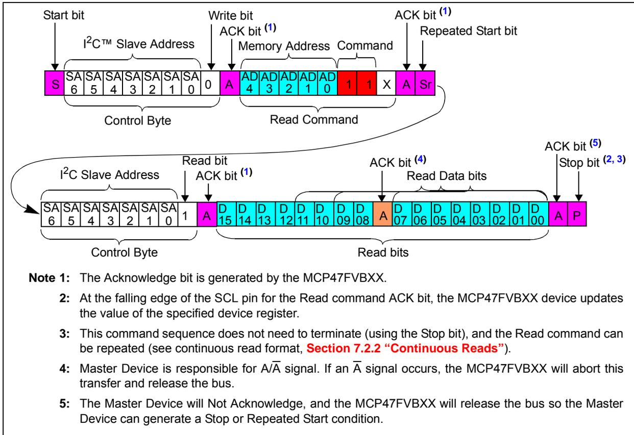
**FIGURE 7-4:** Read Command - Single Memory Address.
