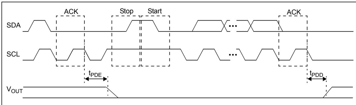
**FIGURE 1-3:** I<sup>2</sup>C™ Power-Down Command Timing.
