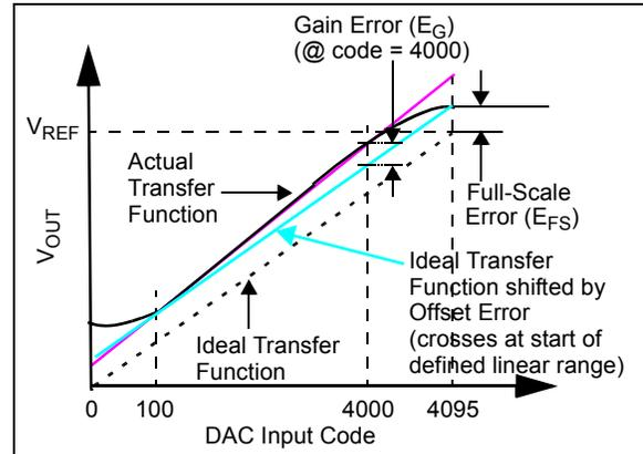
**FIGURE C-3:** Gain Error and Full-Scale Error Example.
