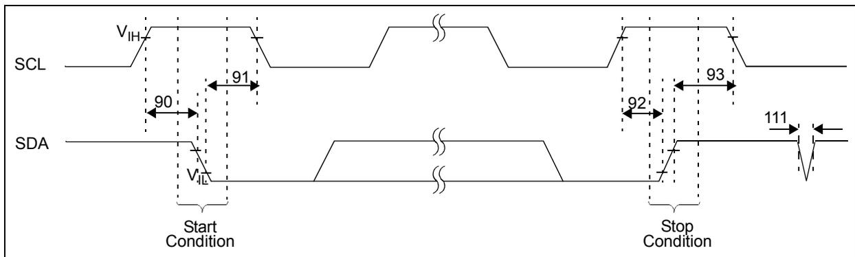
**FIGURE 1-5:**  $I^2C^{TM}$  Bus Start/Stop Bits Timing Waveforms.
