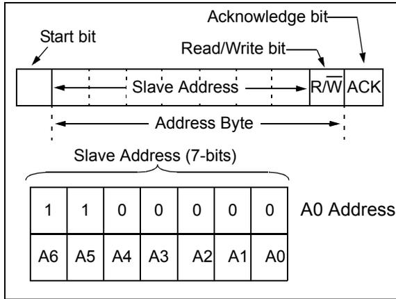
**FIGURE 6-2:** Slave Address Bits in the I<sup>2</sup>C Control Byte.
