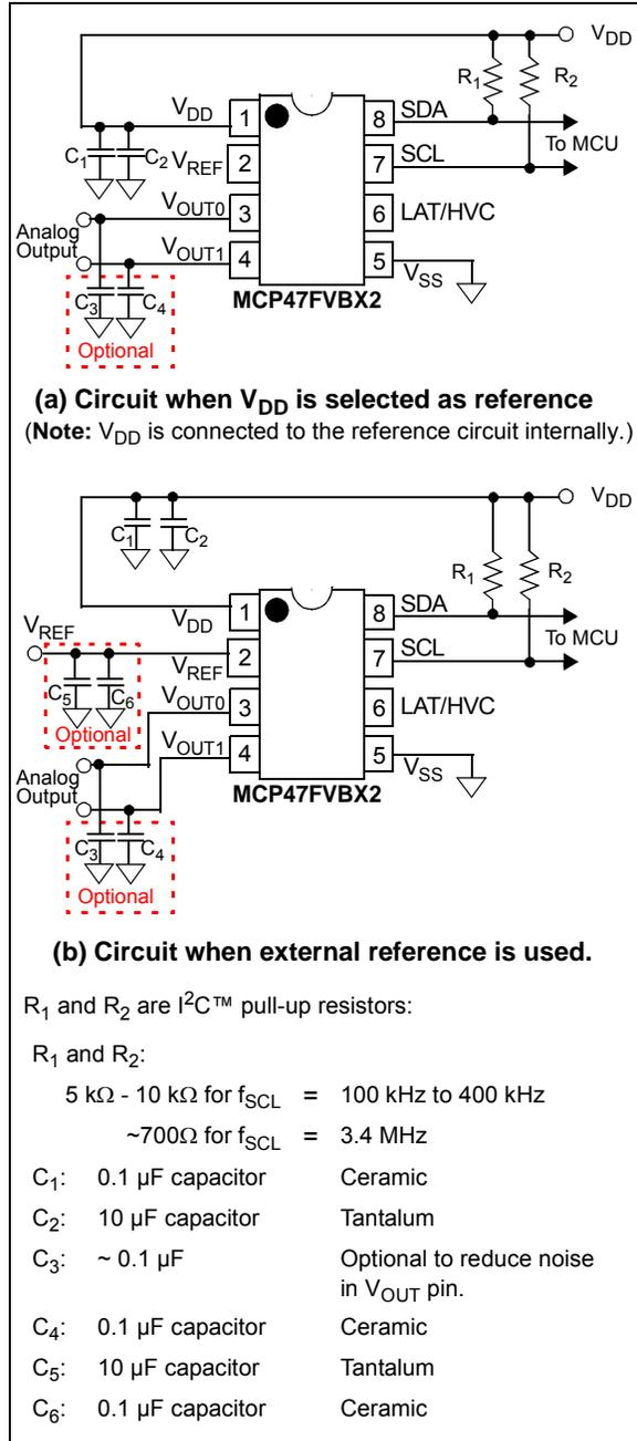
**FIGURE 8-2:** Example Circuit.
