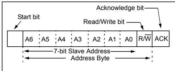
**FIGURE B-9:** I<sup>2</sup>C Slave Address Control Byte.
