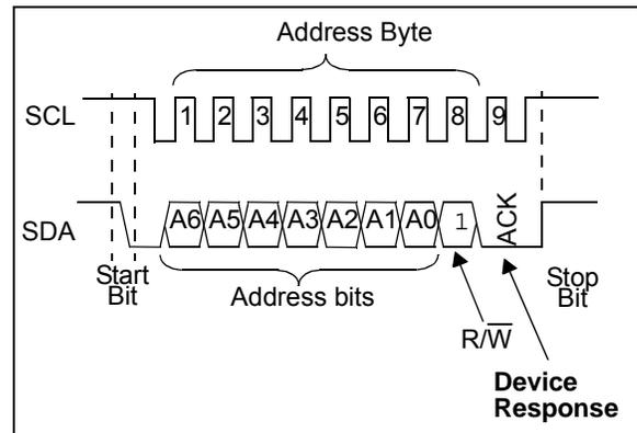
**FIGURE 8-1:** I<sup>2</sup>C Bus Connection Test.
