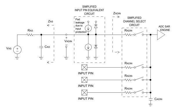
Figure 19. ADC input impedance equivalency diagram
