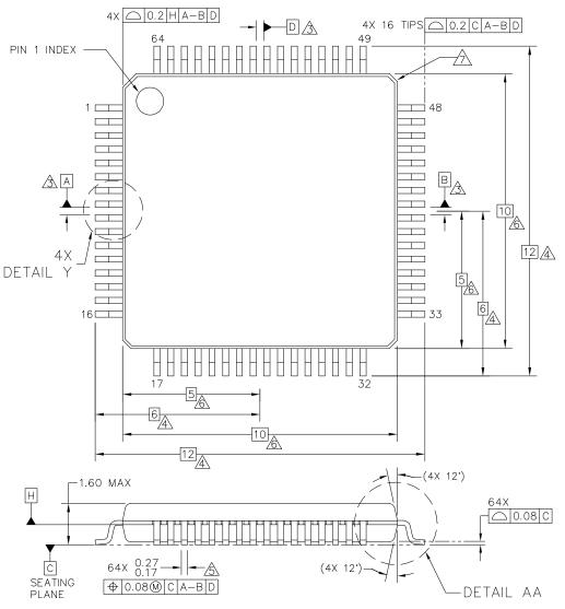
Figure 11. 64-pin LQFP package dimensions 1
