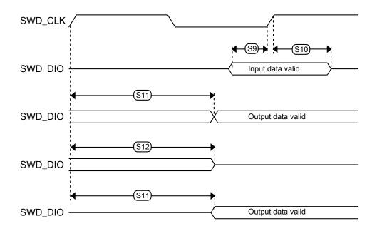
Figure 29. Serial wire data timing
