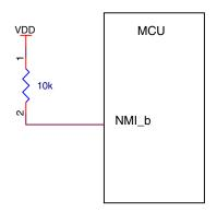
Figure 34. NMI pin biasing
