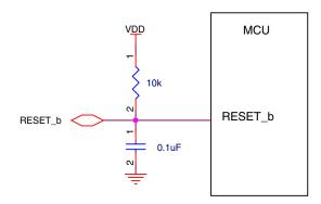
Figure 32. Reset circuit
