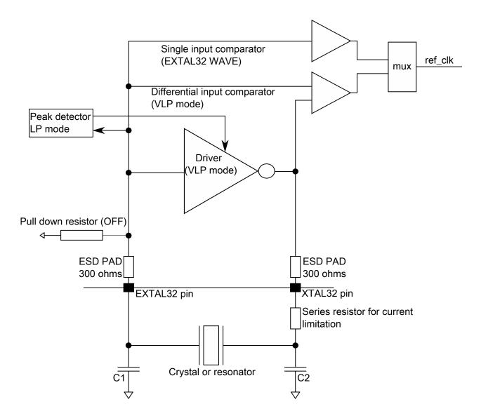
Figure 17. Oscillator connections scheme (OSC32)
