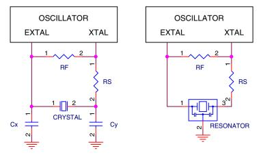
Figure 38. Crystal connection – Diagram 3
