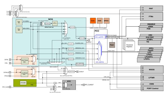
Figure 4. Clocking block diagram
