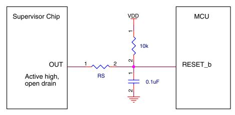
Figure 33. Reset signal connection to external reset chip
