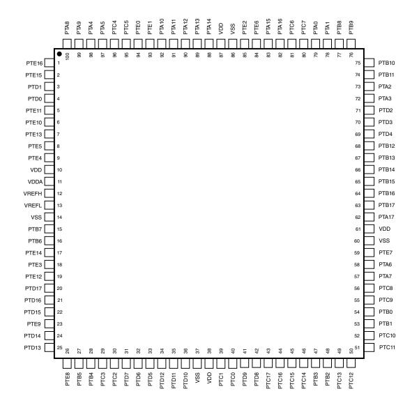
Figure 7. 100 LQFP Pinout Diagram
