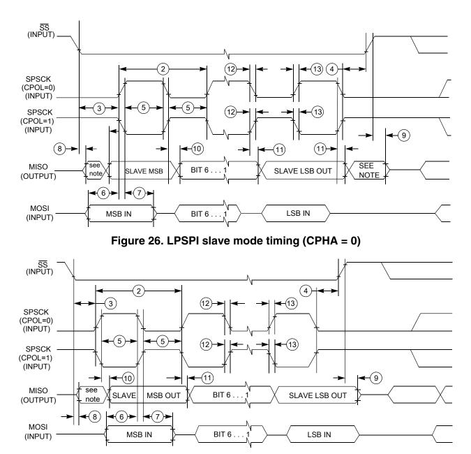
Figure 27. LPSPI slave mode timing (CPHA = 1)
