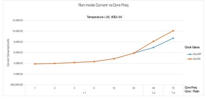
Figure 14. Run mode supply current vs. core frequency
