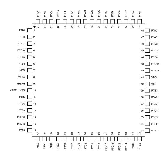
Figure 8. 64 LQFP Pinout Diagram
