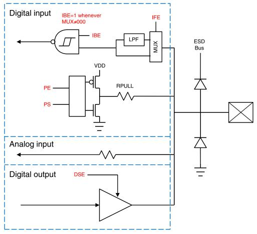
Figure 5. I/O simplified block diagram
