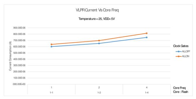
Figure 15. VLPR mode supply current vs. core frequency
