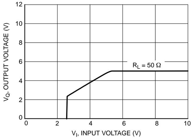
Figure 10. Output Voltage  $V_Q$  vs. Input Voltage  $V_I$
