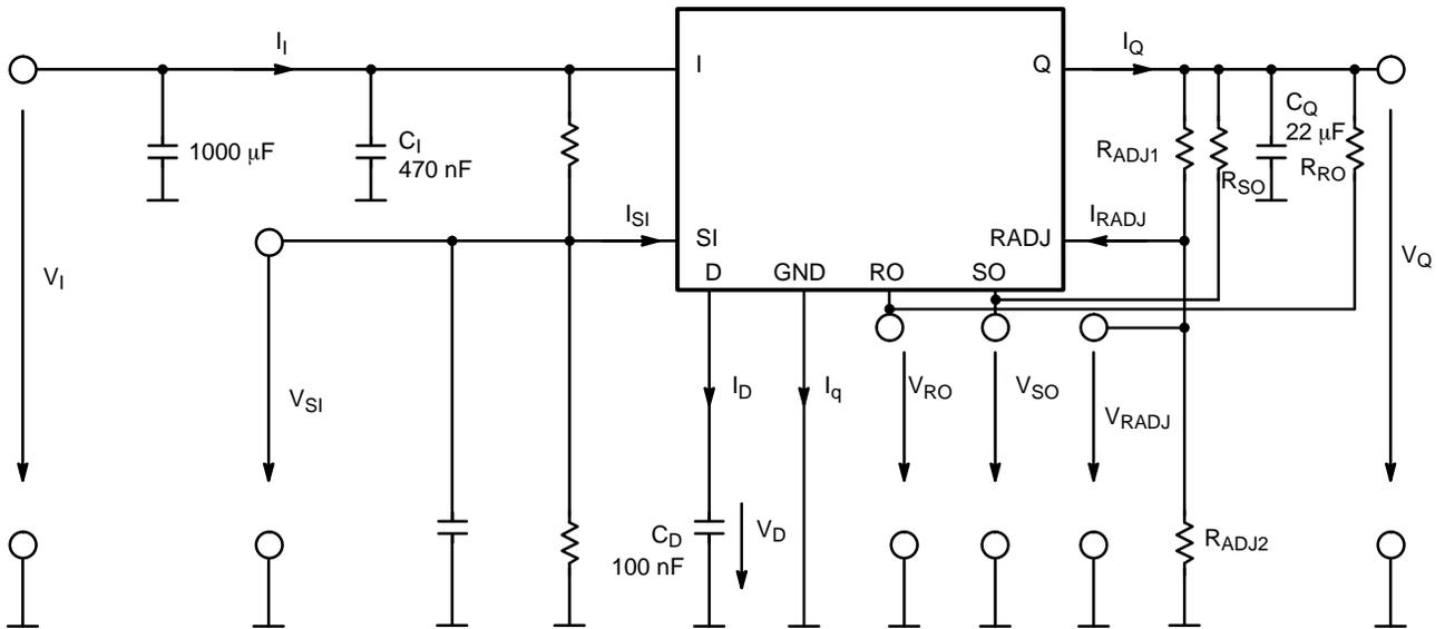
Figure 2. Measuring Circuit
