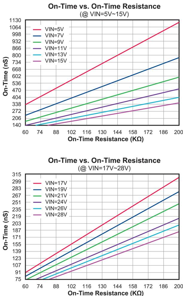
Figure 3.  $T_{ON}$  vs.  $R_{TON}$  Curves for AOZ2262AQI-18
