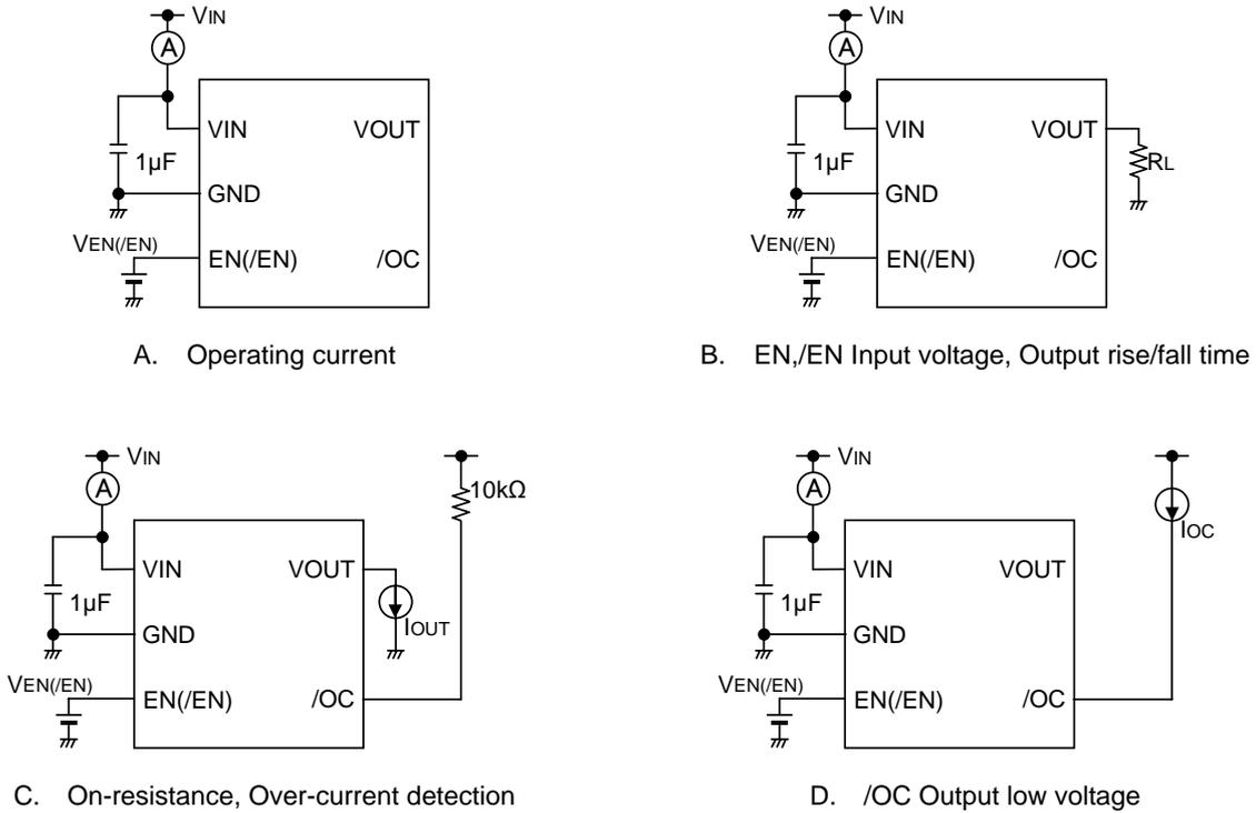
Figure 1. Measurement circuit
