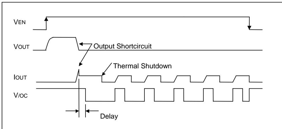
Figure 38. Over-current detection, Thermal shutdown timing (BD2226G)
