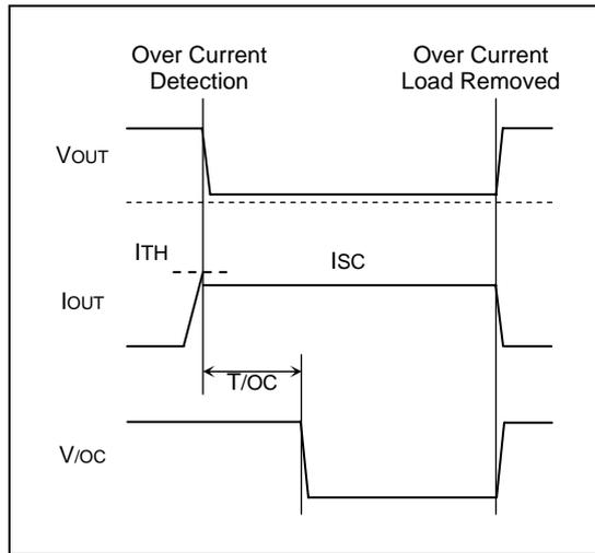
Figure 37. Over-current detection
