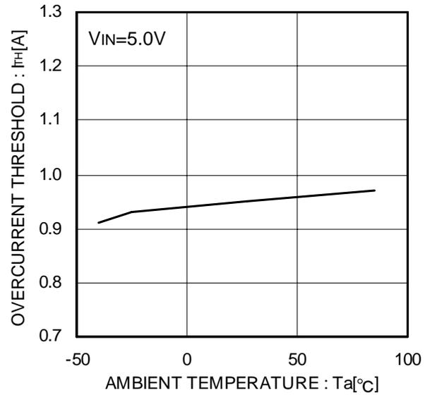
Figure 13. Over-current threshold
