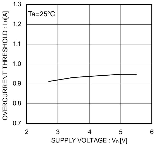
Figure 12. Over-current threshold
