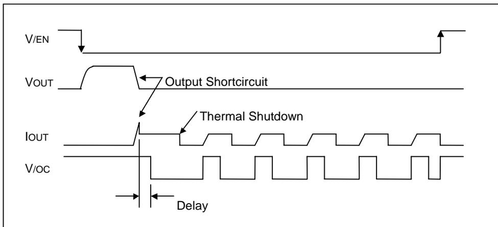
Figure 39. Over-current detection, Thermal shutdown timing (BD2227G)
