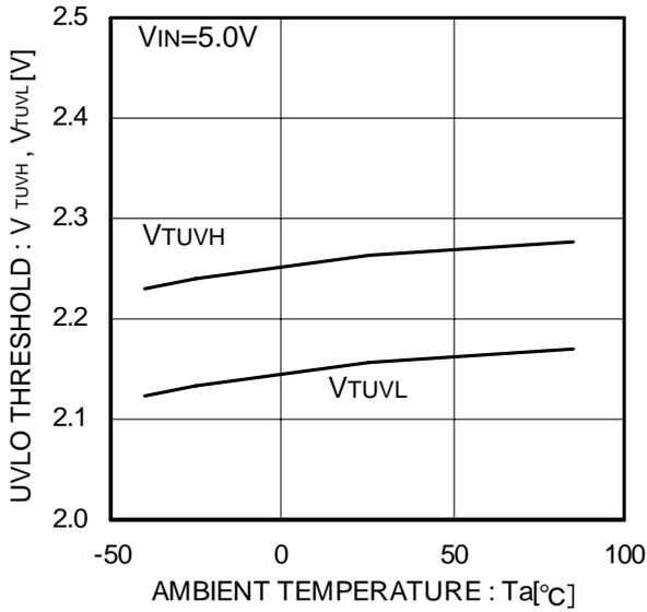
Figure 16. UVLO threshold
