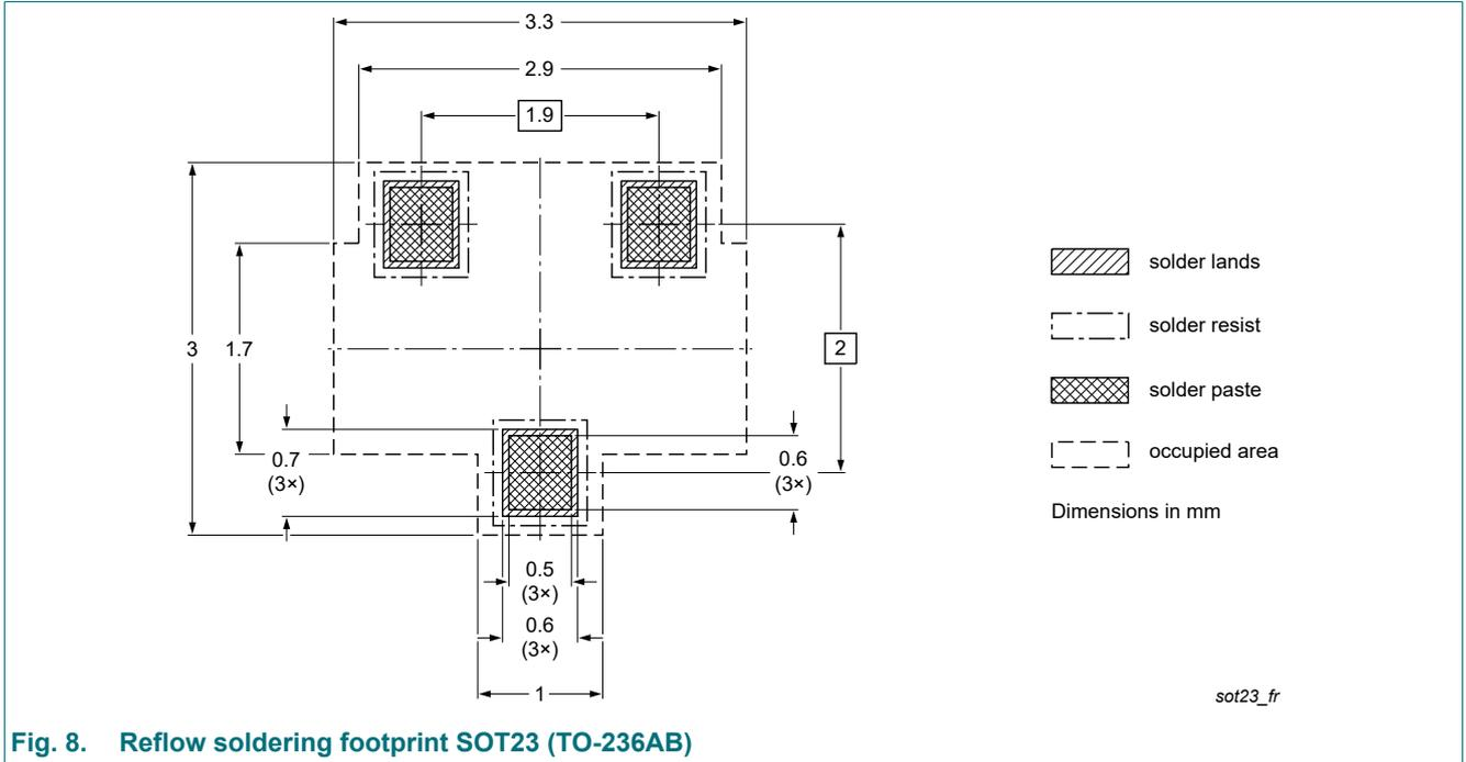
Fig. 8. Reflow soldering footprint SOT23 (TO-236AB)
