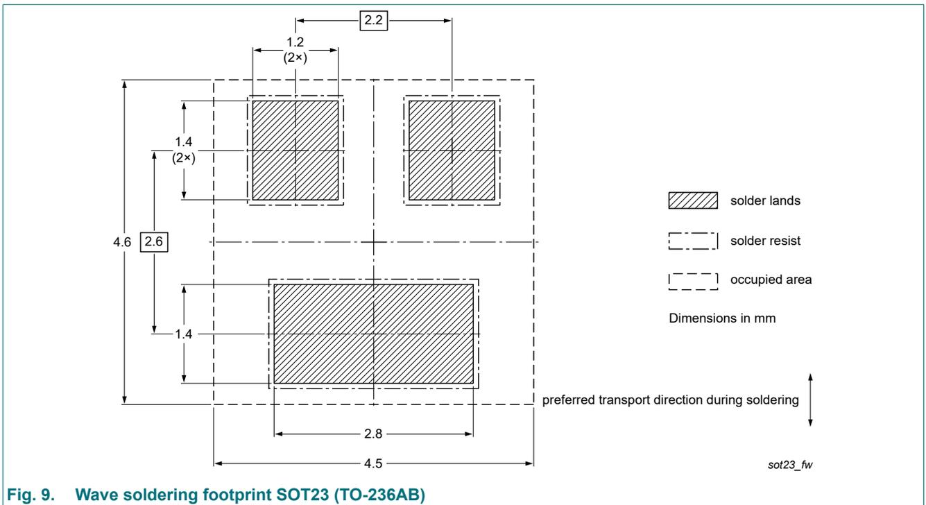
Fig. 9. Wave soldering footprint SOT23 (TO-236AB)
