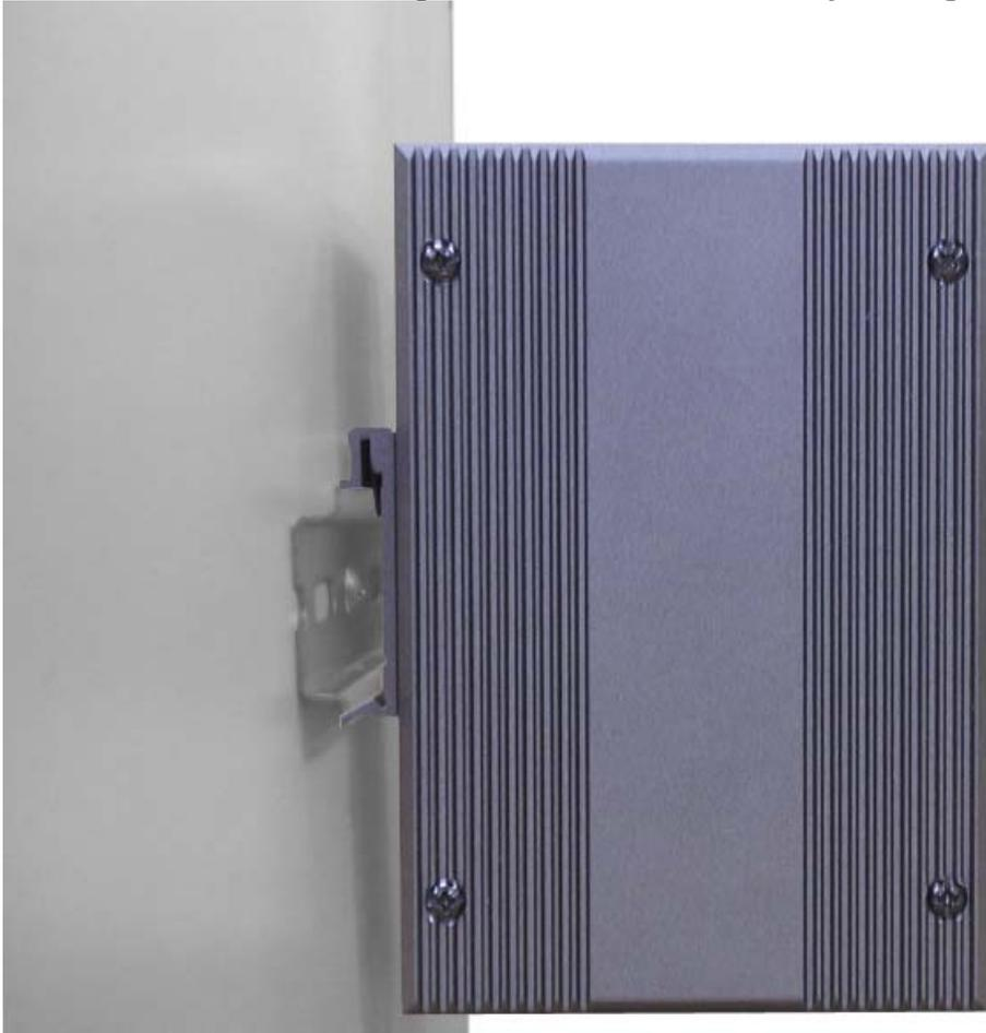
*Figure 2.7: Installation to DIN-rail Step 2*
