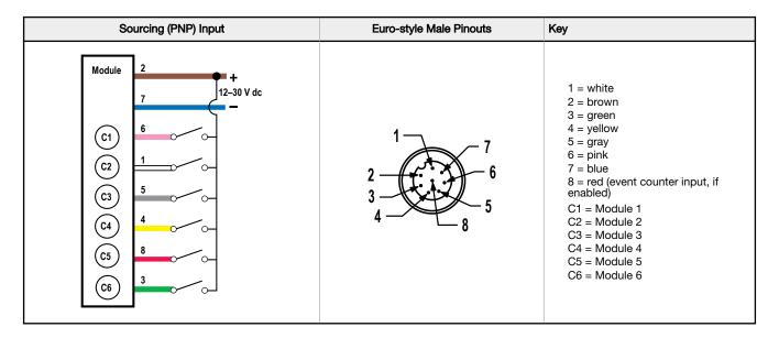
Input wires C1 through C6 can be used to either control the light segments or can be configured as external PNP Inputs. Refer to the DIP switch settings for configuration instructions.
