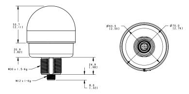
All measurements are listed in millimeters [inches], unless noted otherwise. Dimensions for the quick disconnect model are shown.
