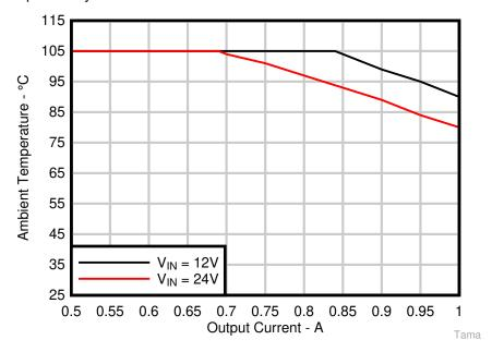
Figure 9-2. Maximum Output Current versus Ambient Temperature
