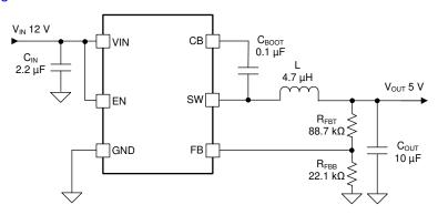
Figure 9-1. Application Circuit
