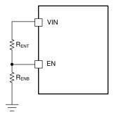
Figure 8-3. System UVLO by Enable Divider
