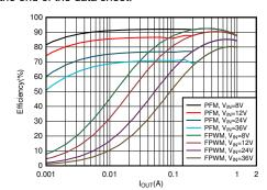
Efficiency versus Output Current  $V_{OUT} = 5 V$ , 2.1MHz
