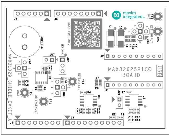
MAX31329 Shield PCB Layout Diagram—Top Silkscreen
