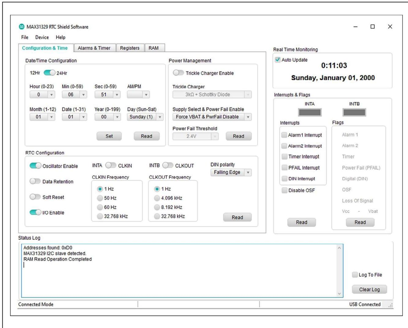
Figure 2. MAX31329 RTC Shield Software—Configuration and Time Page
