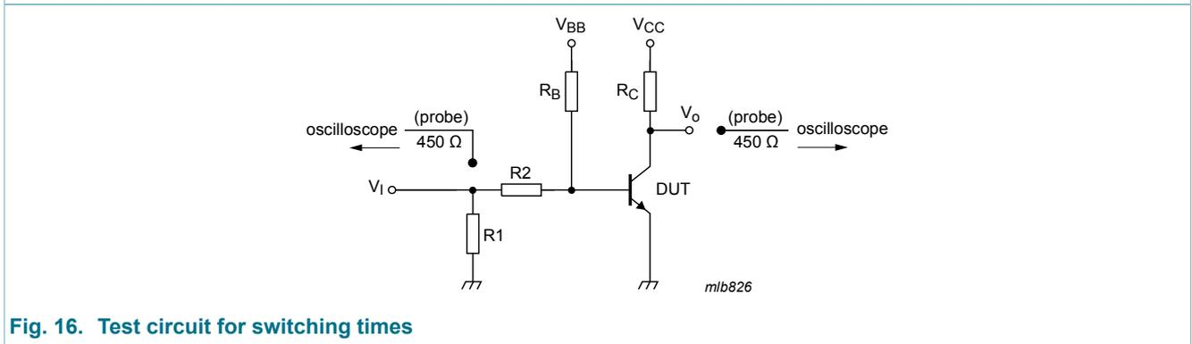
Fig. 16. Test circuit for switching times
