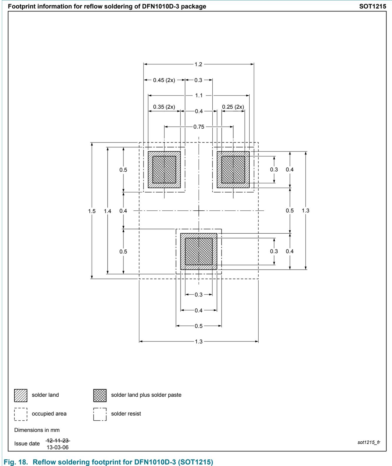
Fig. 18. Reflow soldering footprint for DFN1010D-3 (SOT1215)
