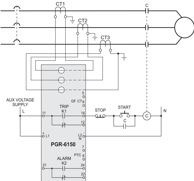
For motors with nominal current over the maximum relay current set-point value, combine the relay with current transformers. Set the value  $I_B$  and CT Turns Ratio as explained in Section 6.2.1.
