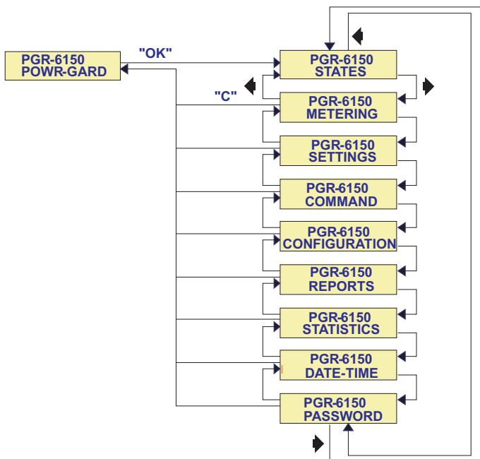
Press the “OK” key to access the first level from the main screen. Use the “◀” and “▶” keys to move from one menu section to another in the first level. Use the “C” key to return to a higher level.
