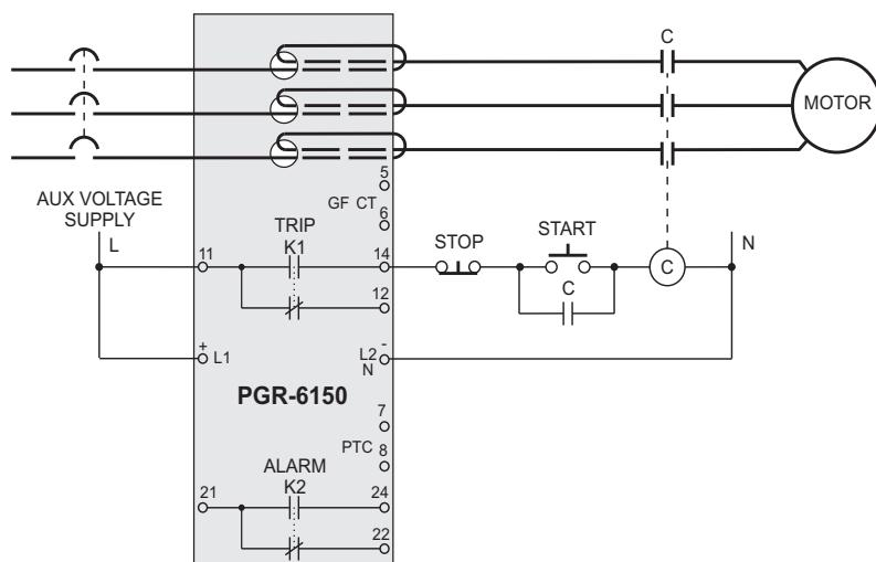
For motors with nominal current below the minimum relay set-point value, multiple turns can be used. Set the value  $I_B$  and CT Turns Ratio as explained in Section 6.2.1.
