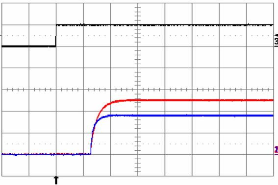
**Fig. 18:** Turn-on transient waveforms at no load current and  $V_{in} = 48\text{ V}$ , triggered via ON/OFF pin. Top trace: ON/OFF signal (5 V/div.). Bottom traces:  $V_{out1}$  (blue, 1 V/div.),  $V_{out2}$  (red, 1 V/div.). Time scale: 1 ms/div.
