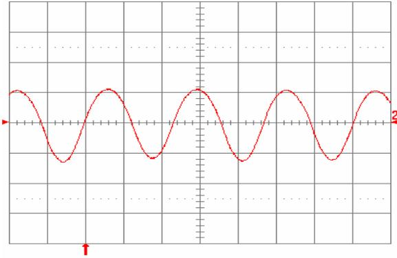
**Fig. 32:** Input reflected ripple current,  $i_c$  (100 mA/div), measured at input terminals at full rated load current on both outputs and  $V_{in} = 48$  V. Refer to Fig. 31 for test setup. Time scale: 1  $\mu$ s/div.
