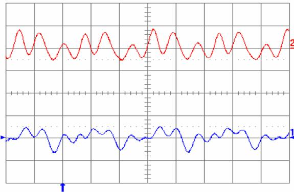
**Fig. 30:** Output voltage ripple at full rated load current into a resistive load on both outputs with  $C_o = 1\mu\text{F}$  (ceramic) and  $V_{in} = 48\text{ V}$ . Ch2 =  $V_{out2}$ , Ch1 =  $V_{out1}$  (both 20 mV/div). Time scale:  $1\text{ }\mu\text{s/div}$ .
