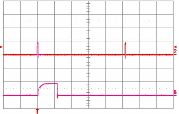
**Fig. 29:** Load current  $i_{out2}$  into a  $10\text{ m}\Omega$  short circuit on  $V_{out2}$  during restart, with  $V_{out1}$  open (no load), at  $V_{in} = 48\text{ V}$ . Ch2 =  $i_{out2}$  (20 A/div, 20 ms/div). ChB =  $i_{out2}$  (20 A/div, 1 ms/div) is an expansion of the on-time portion of  $i_{out2}$ .
