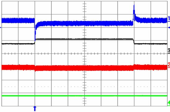
**Fig. 20:** Output voltage response to Iout1 load current step-change of 3.75 A (50%-75%-50%) at Iout2 = 7.5 A and Vin = 48 V. Ch1 = Vout1 (50 mV/div), Ch2 = Vout2 (50 mV/div), Ch3 = Iout1 (10 A/div.), Ch4 = Iout2 (10 A/div.). Current slew rate: 0.1 A/μs, Co = 10 μF tantalum + 1 μF ceramic. Time scale: 0.5 ms/div.
