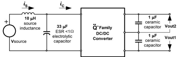
**Fig. 31:** Test setup for measuring input reflected ripple currents,  $i_c$  and  $i_s$ .
