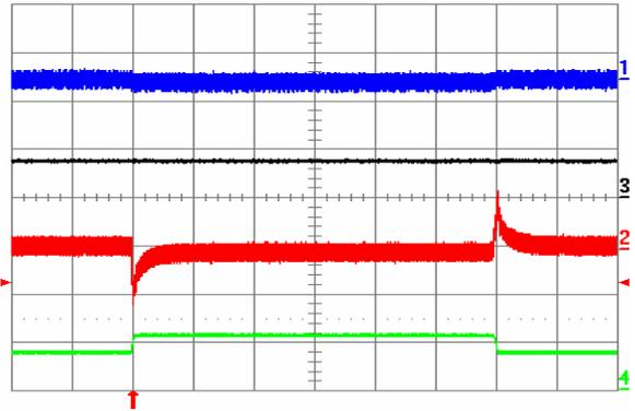
**Fig. 21:** Output voltage response to Iout2 load current step-change of 3.75 A (50%-75%-50%) at Iout1 = 7.5 A and Vin = 48 V. Ch1 = Vout1 (50 mV/div), Ch2 = Vout2 (50 mV/div), Ch3 = Iout1 (10 A/div.), Ch4 = Iout2 (10 A/div.). Current slew rate: 0.1 A/μs, Co = 10 μF tantalum + 1 μF ceramic. Time scale: 0.5 ms/div.
