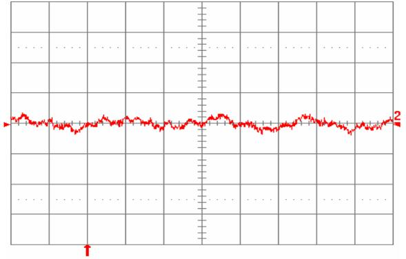
**Fig. 33:** Input reflected ripple current,  $i_s$  (10 mA/div), measured through 10  $\mu$ H at the source at full rated load current on both outputs and  $V_{in} = 48$  V. Refer to Fig. 31 for test setup. Time scale: 1  $\mu$ s/div.
