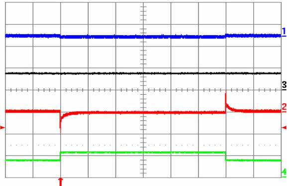
**Fig. 23:** Output voltage response to Iout2 load current step-change of 3.75 A (50%-75%-50%) at Iout1 = 7.5 A and Vin = 48 V. Ch1 = Vout1 (100 mV/div), Ch2 = Vout2 (100 mV/div), Ch3 = Iout1 (10 A/div.), Ch4 = Iout2 (10 A/div.). Current slew rate: 5 A/μs, Co = 300 μF tantalum + 1 μF ceramic. Time scale: 0.5 ms/div.
