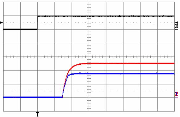
**Fig. 19:** Turn-on transient waveforms at full rated load current (resistive) and  $V_{in} = 48\text{ V}$ , triggered via ON/OFF pin. Top trace: ON/OFF signal (5 V/div.). Bottom traces:  $V_{out1}$  (blue, 1 V/div.),  $V_{out2}$  (red, 1 V/div.). Time scale: 1 ms/div.
