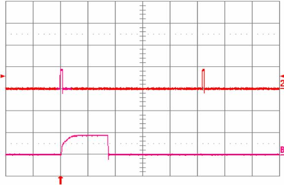
**Fig. 28:** Load current  $i_{out1}$  into a  $10\text{ m}\Omega$  short circuit on  $V_{out1}$  during restart, with  $V_{out2}$  open (no load), at  $V_{in} = 48\text{ V}$ . Ch2 =  $i_{out1}$  (20 A/div, 20 ms/div). ChB =  $i_{out1}$  (20 A/div, 1 ms/div) is an expansion of the on-time portion of  $i_{out1}$ .
