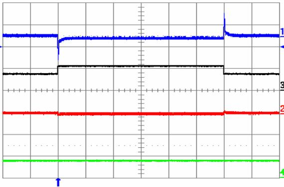
**Fig. 22:** Output voltage response to Iout1 load current step-change of 3.75 A (50%-75%-50%) at Iout2 = 7.5 A and Vin = 48 V. Ch1 = Vout1 (100 mV/div), Ch2 = Vout2 (100 mV/div), Ch3 = Iout1 (10 A/div.), Ch4 = Iout2 (10 A/div.). Current slew rate: 5 A/μs, Co = 300 μF tantalum + 1 μF ceramic. Time scale: 0.5 ms/div.
