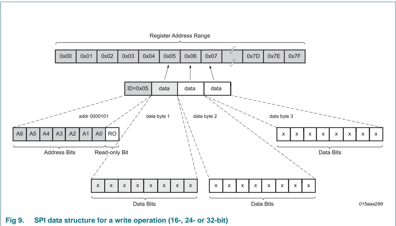
Fig 9. SPI data structure for a write operation (16-, 24- or 32-bit)
