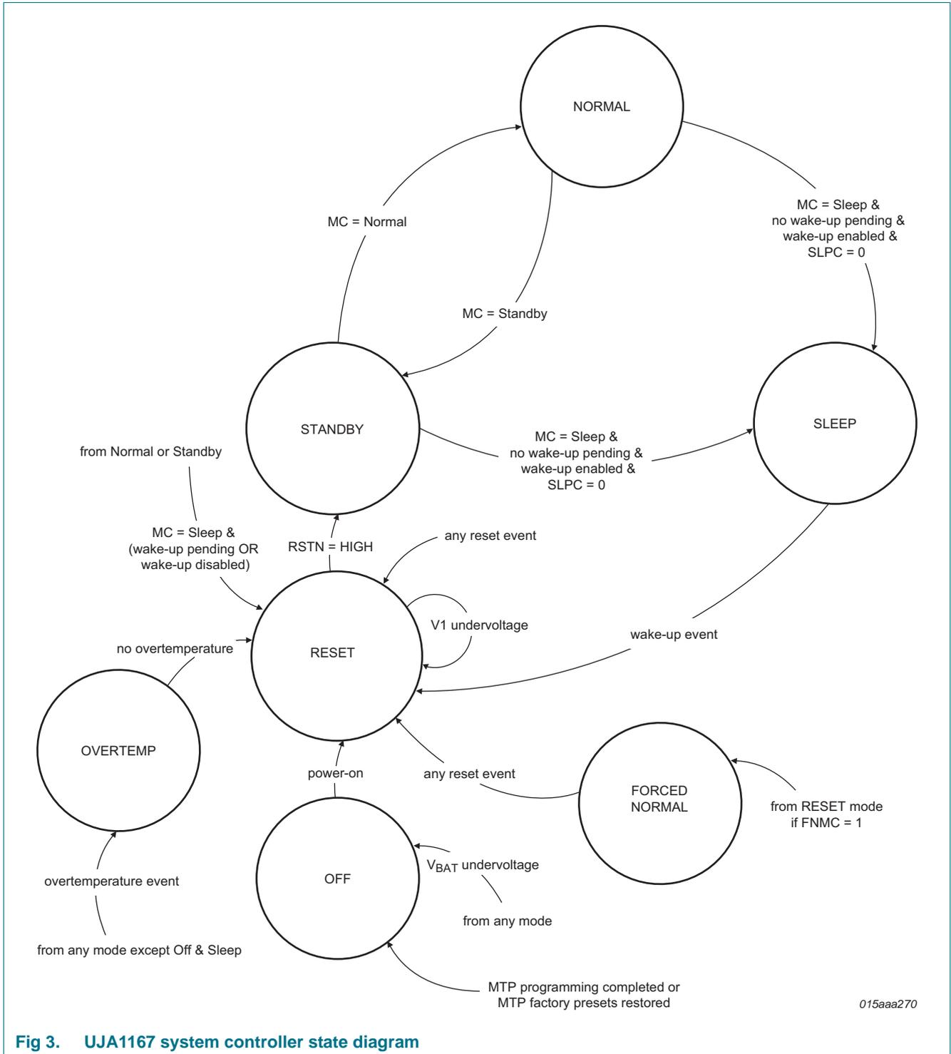
Fig 3. UJA1167 system controller state diagram
