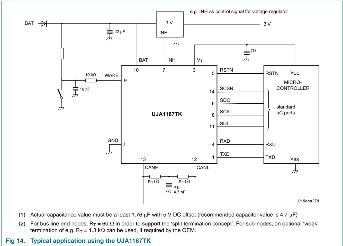
Fig 14. Typical application using the UJA1167TK
