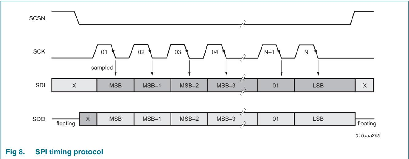
Fig 8. SPI timing protocol
