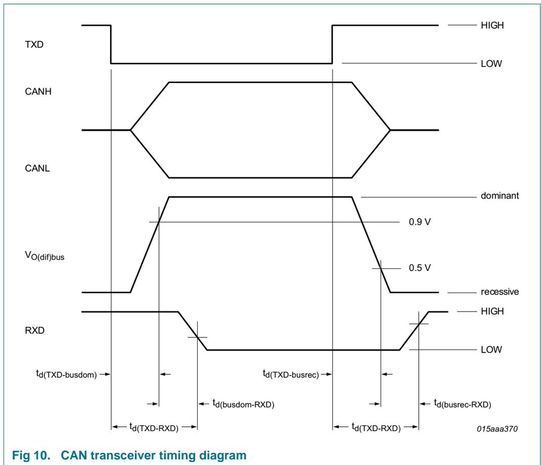
**Fig 10. CAN transceiver timing diagram**
