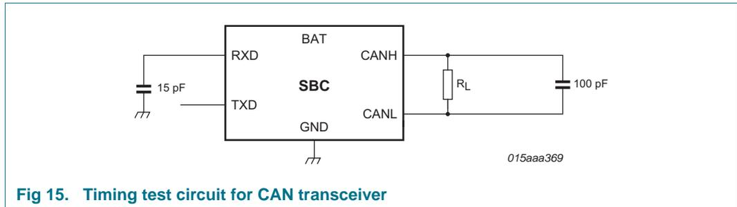
Fig 15. Timing test circuit for CAN transceiver
