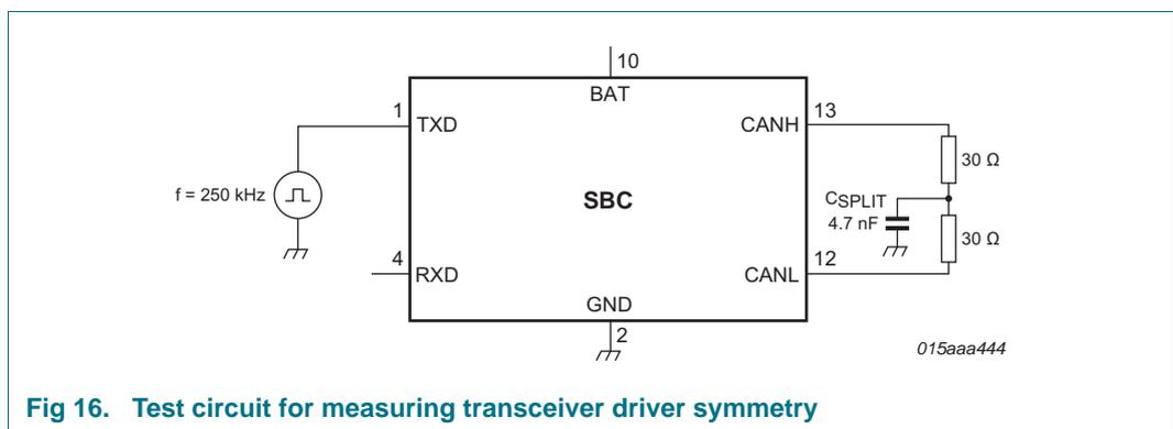
Fig 16. Test circuit for measuring transceiver driver symmetry
