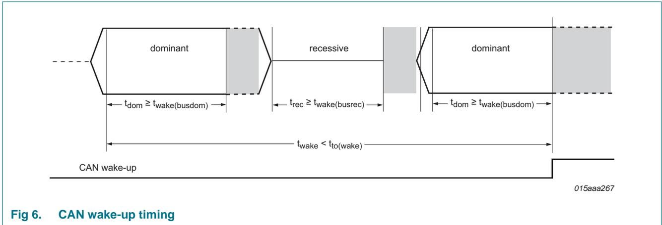
Fig 6. CAN wake-up timing
