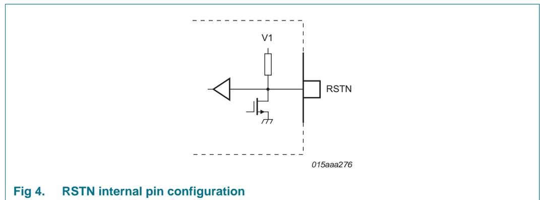
**Fig 4. RSTN internal pin configuration**
