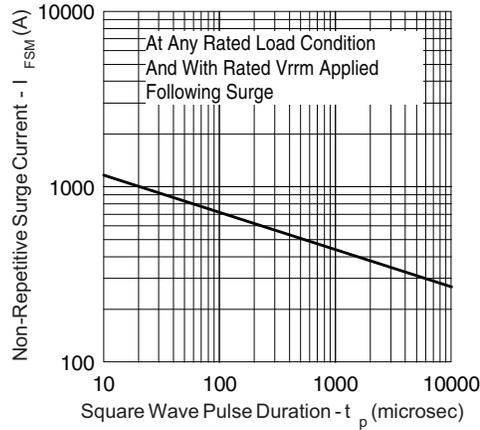
Fig. 7 - Maximum Non-Repetitive Surge Current (Per Leg)
