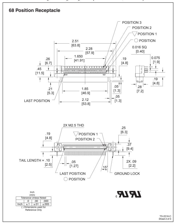
.050" Boardmount Through-Hole Right Angle Receptacle - Shielded, SCSI-2 Layout 102 Series
