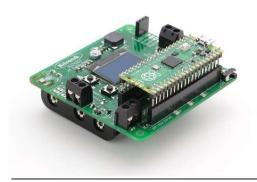
The 'POWER' terminal block can also be used as the connection point for a solar cell. **NOTE:** Please ensure the correct rechargeable batteries are fitted before charging, they should be **NiMh**.
