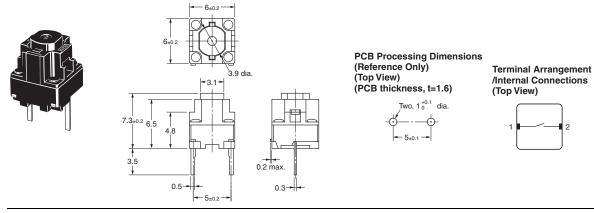
Note: Unless otherwise specified, a tolerance of ±0.4 mm applies to all dimensions. No terminal numbers are indicated on the Switches.
