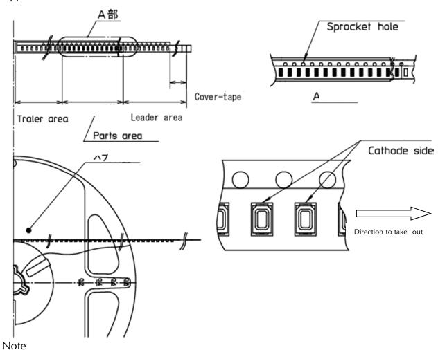
"-TR" means cathode side of LEDs should be placed on the sprocket-hole side.
