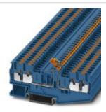
Knife disconnect terminal block, Connection type: Push-in connection, Cross section: 0.14 mm² - 4 mm², AWG: 26 - 12, Nominal current: 16 A, Nominal voltage: 400 V, Length: 92.2 mm, Width: 5.2 mm, Color: blue, Assembly: NS 35/7,5, NS 35/15
