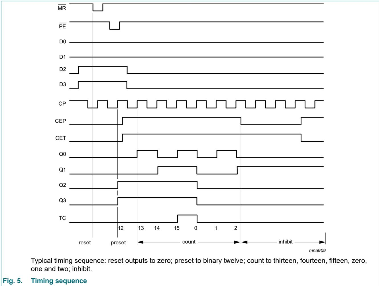
Presettable synchronous 4-bit binary counter; asynchronous reset
