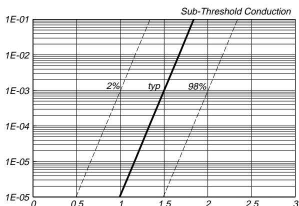
Fig.11. Sub-threshold drain current.
