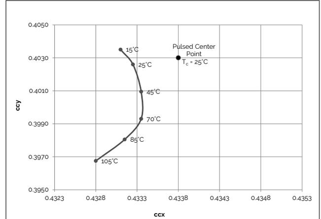
**Figure 13: 3000K, 90 CRI Color Shift vs. Case Temperature<sup>1,3</sup>**
