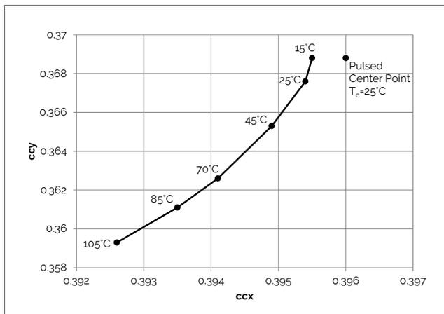
**Figure 16: 4000K Class A Color Shift vs. Case Temperature<sup>1</sup>**
