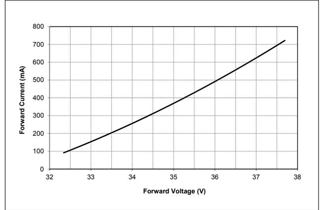
**Figure 3: Vero SE 10D Drive Current vs. Voltage**
