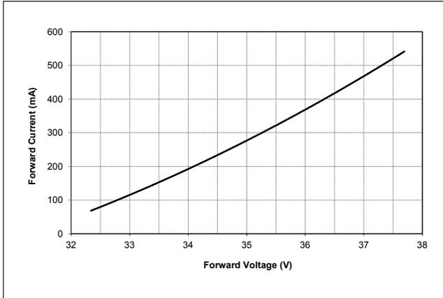
**Figure 2: Vero SE 10C Drive Current vs. Voltage**
