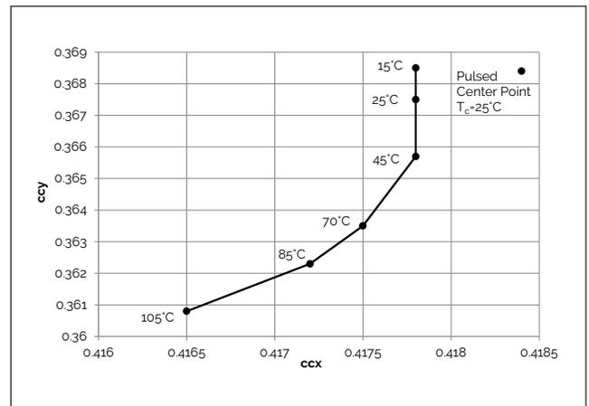
**Figure 15: 3500K Class A Color Shift vs. Case Temperature<sup>1</sup>**
