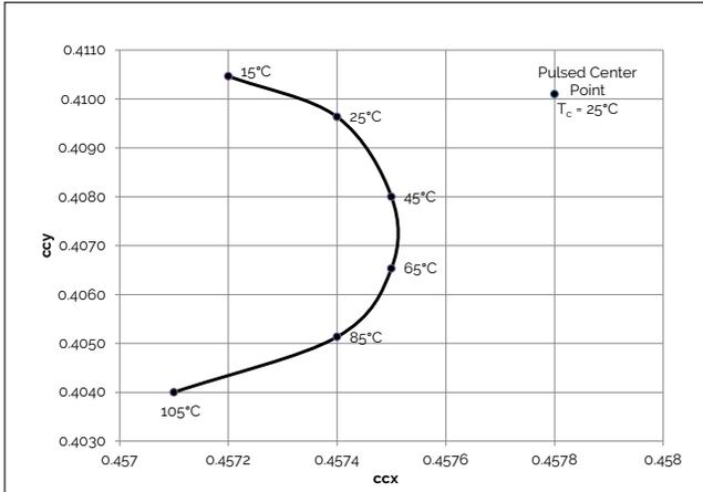
**Figure 12: 3000K, 97 CRI Color Shift vs. Case Temperature<sup>1</sup>**
