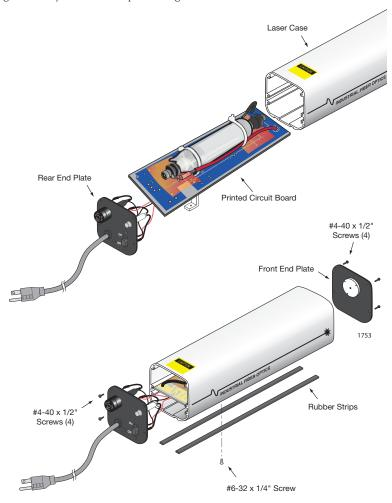
Figure 5. Inserting laser in case.
