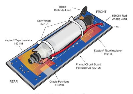
Figure 3. Laser tube mounting diagram.
