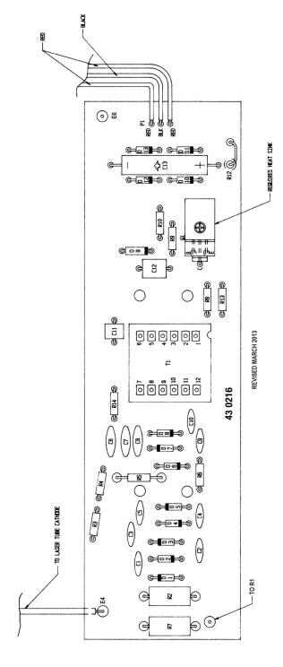
Figure 1. Printed circuit board assembly diagram.
