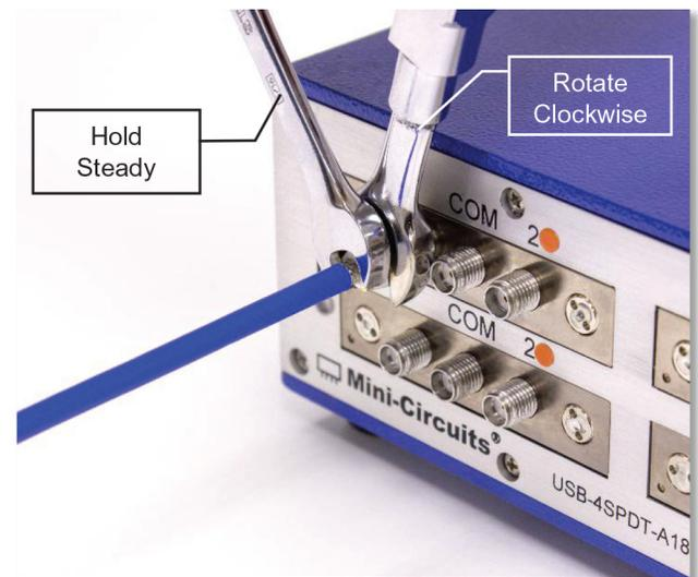
3) Using a 5/16-inch open end wrench, rotate the coupling nut clockwise to tighten the cable connector.
