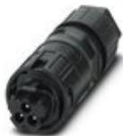
Installation connector, Range of articles: PRC 35, Connector, housing material: PPE, color: black, number of positions: 3, min. conductor cross section: 1.5 mm<sup>2</sup>, max. conductor cross section: 6 mm<sup>2</sup>, nom. voltage: 690 V AC, rated current: 35 A, Connection method: Screw connection, Type of contact: Pin, min. cable diameter: 8 mm, max. cable diameter: 21 mm
