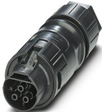
Installation connector, Range of articles: PRC 35, Coupler connector, type: Can only be released with a tool, housing material: PPE, color: black, number of positions: 3, min. conductor cross section: 1.5 mm<sup>2</sup>, max. conductor cross section: 6 mm<sup>2</sup>, nom. voltage: 690 V AC, rated current: 35 A, Connection method: Screw connection, Type of contact: Socket, min. cable diameter: 12 mm, max. cable diameter: 21 mm. Variant for release with a tool
