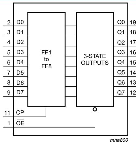
Fig. 3. Functional diagram
