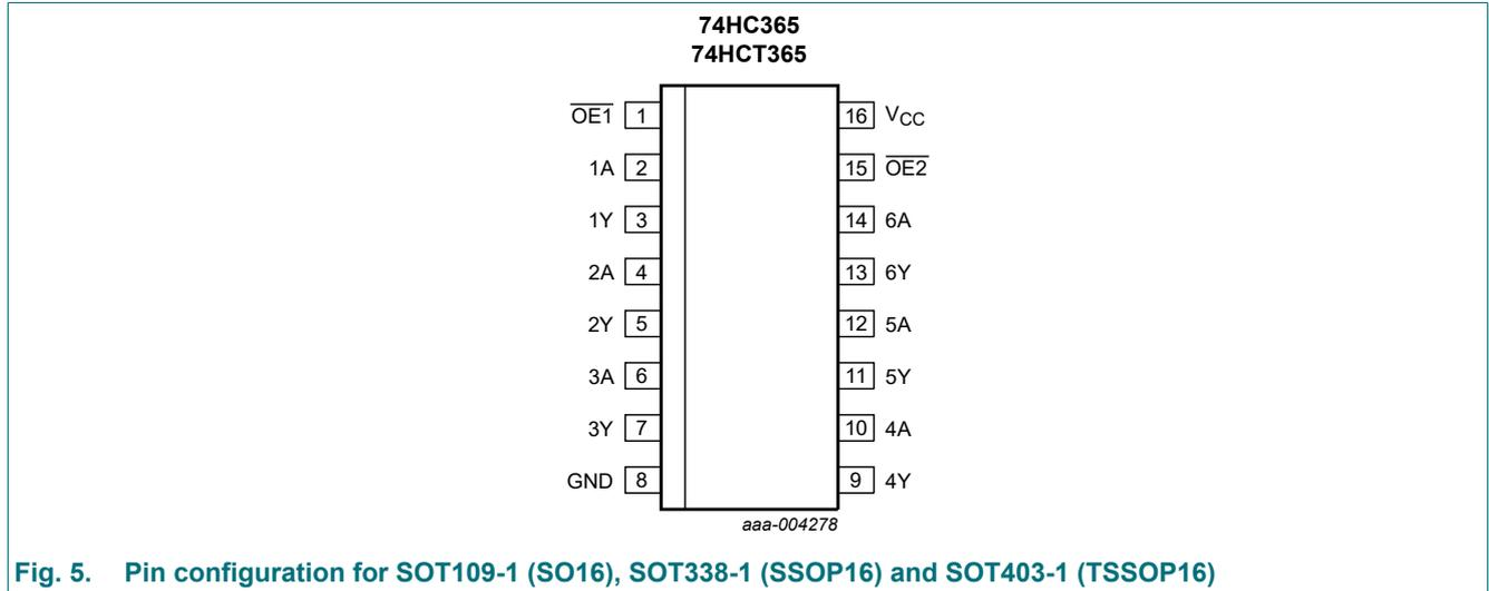
Fig. 5. Pin configuration for SOT109-1 (SO16), SOT338-1 (SSOP16) and SOT403-1 (TSSOP16)
