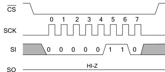
**WRDI - Reset Write Enable Latch**
