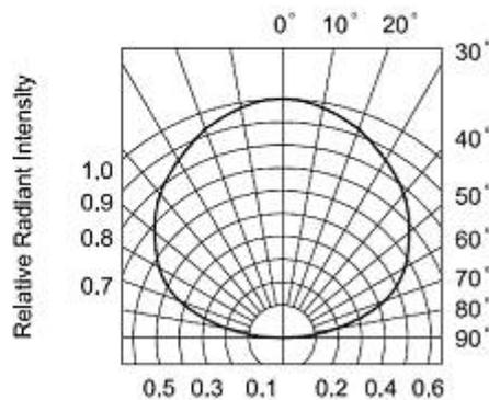
FIG.6 RADIATION DIAGRAM
