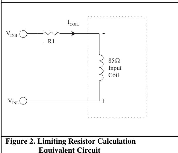
**Figure 2. Limiting Resistor Calculation Equivalent Circuit**
