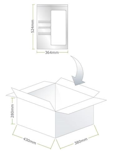
Pallet Dimensions: 1200mm\*1000mm\*1280mm 24 Cartons per Pallet 6 Cartons per Layer, 4 Layers
