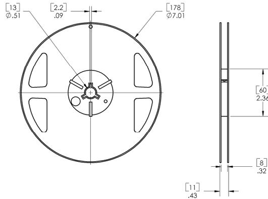
Carrier Tape Dimensions: Loaded quantity 2000 pieces per reel
