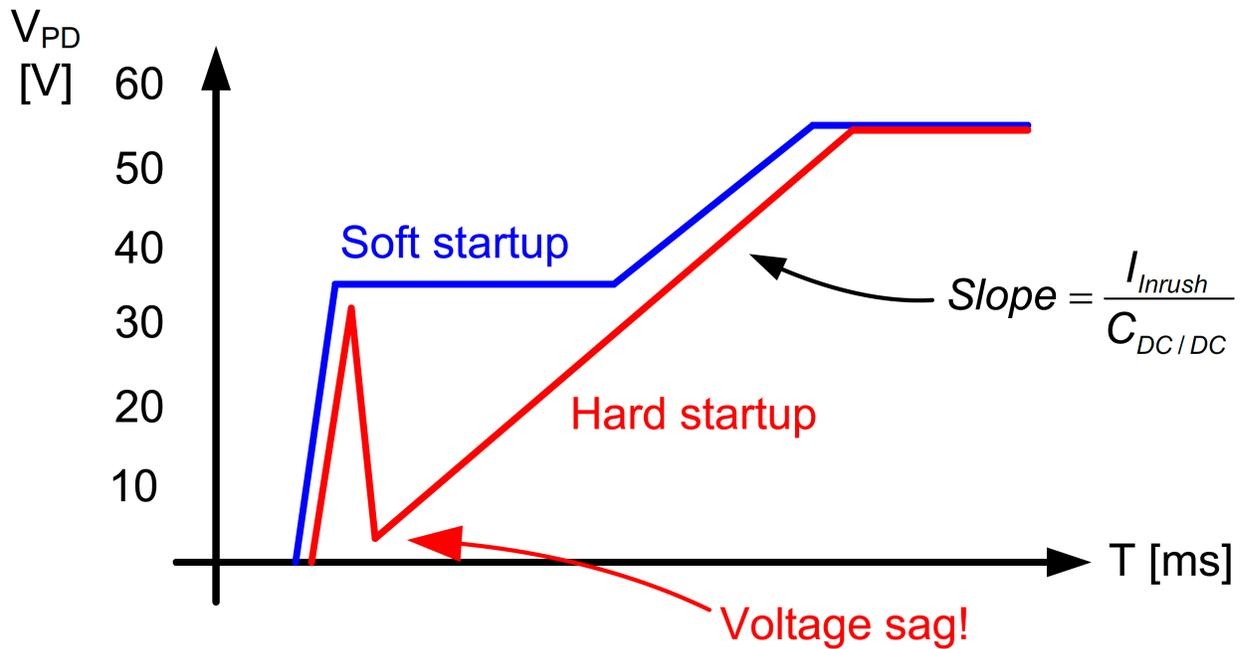
Once bulk capacitance has charged up to a point where  $VPN_{OUT}$  to  $VPN_{IN}$  differential voltage is less than 0.7 V, the isolation MOSFET is switched into normal operating mode with MOSFET current limit set at 1.8 A (typical), to provide over-current protection.
