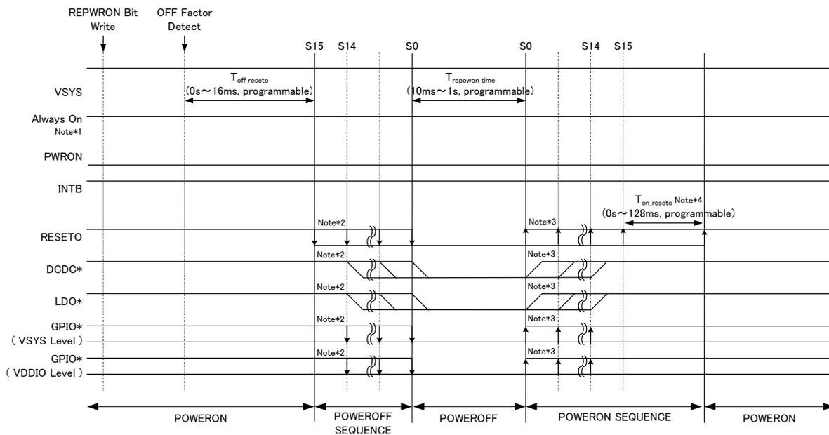
Fig. 6-6 Repower-on Sequence
