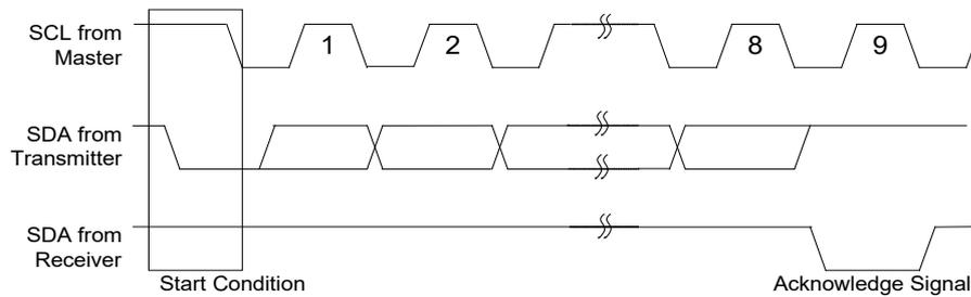
Fig. 10-4 I<sup>2</sup>C-Bus Data Transmission and Acknowledge
