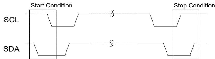
Fig. 10-2 I<sup>2</sup>C-Bus Start and Stop Condition
