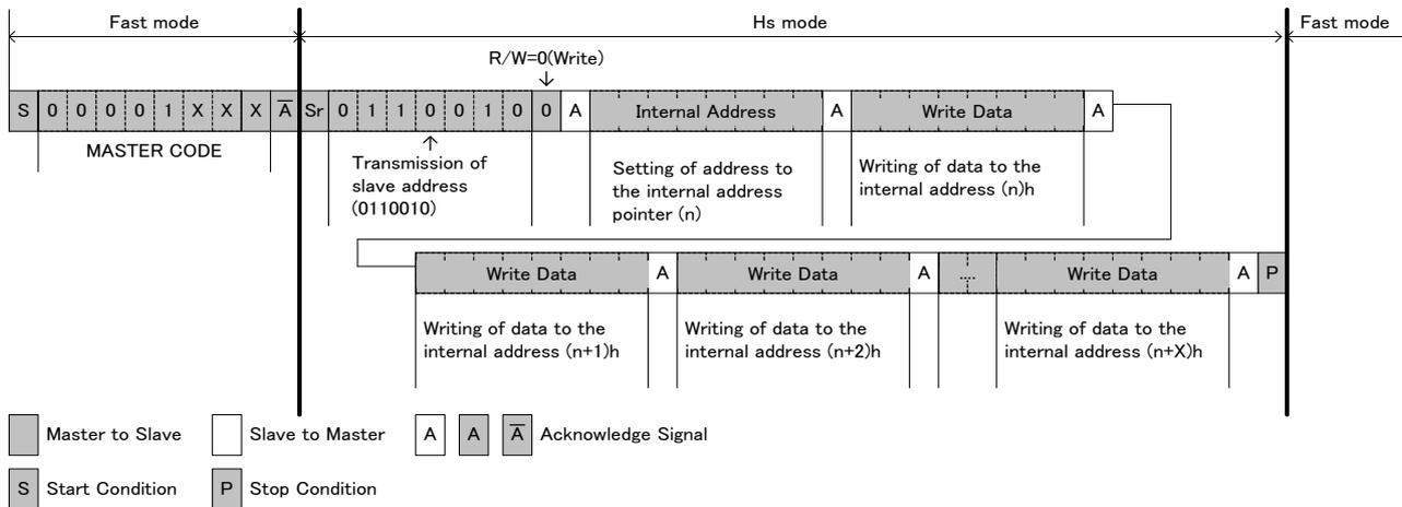
Fig. 10-5 I<sup>2</sup>C-Bus Data Transmission Write Format (Hs-mode)
