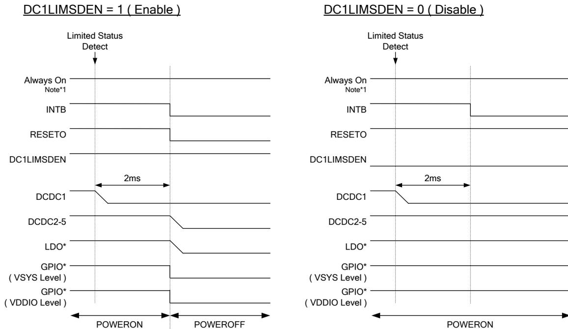
Fig. 6-10 Shutdown Sequence (DCDC1 current limit detection)
