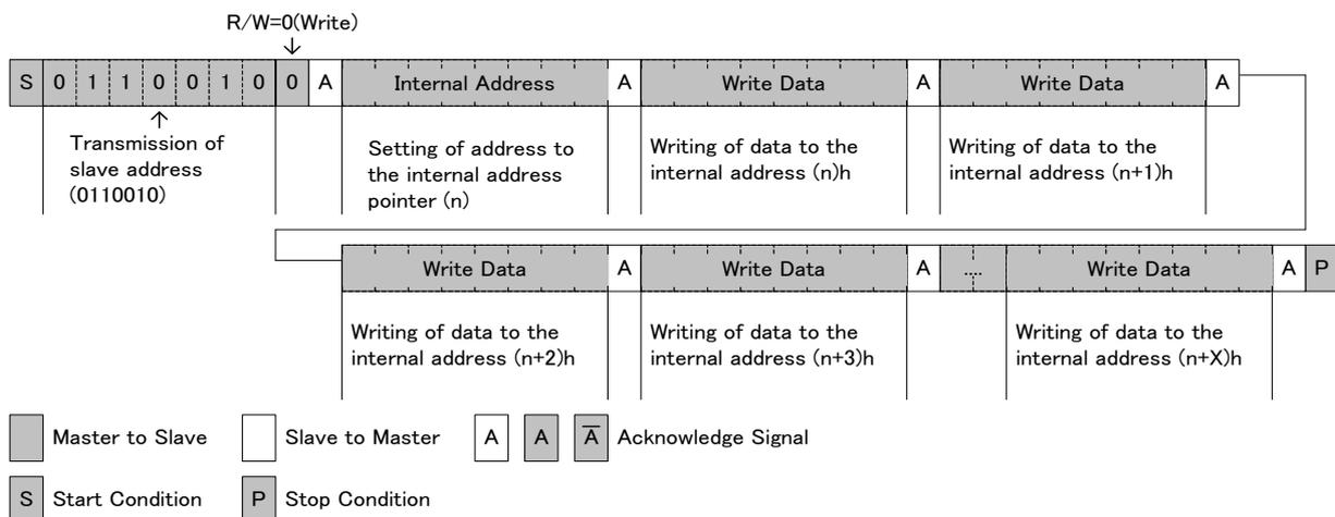
Fig. 10-1 I<sup>2</sup>C-Bus Data Transmission Write Format
