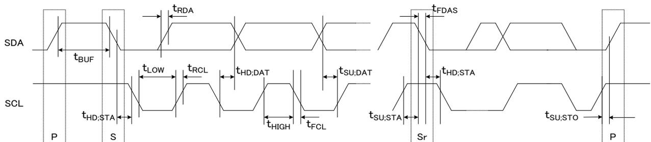
Fig. 10-3 I<sup>2</sup>C-Bus Interface Timing Chart
