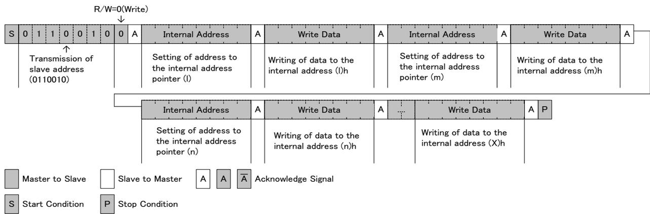
Fig. 10-2 I<sup>2</sup>C-Bus Data Transmission Write Format (Power I<sup>2</sup>C)
