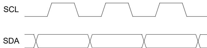
Fig. 10-1 I<sup>2</sup>C-Bus Data Transmission
