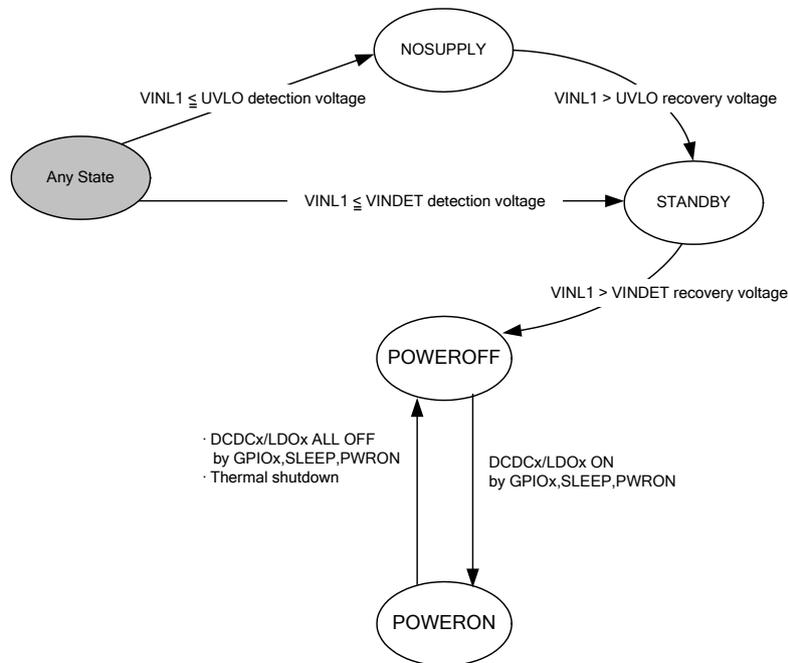
Fig. 8-3 State Machine Diagram in Parts mode
