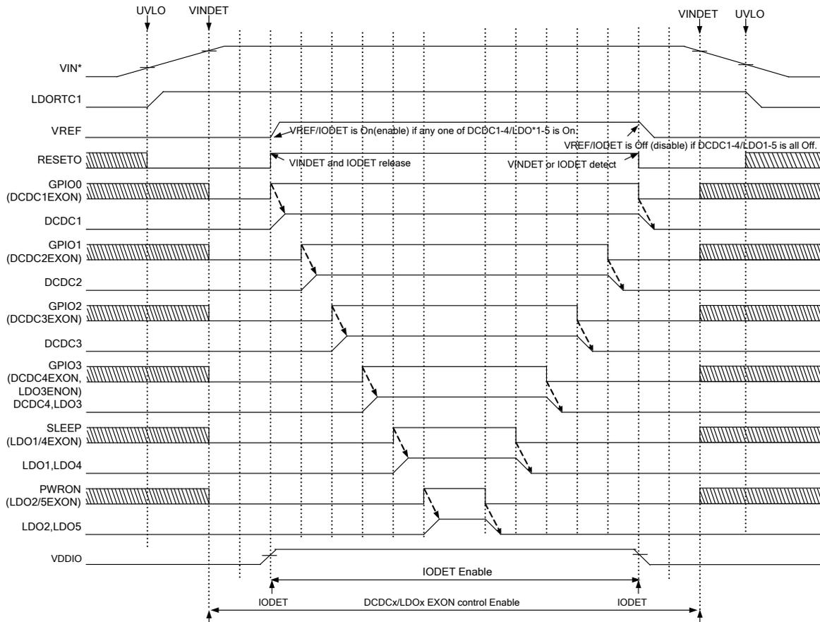
Fig. 8-1 Power On/Off function in Parts mode
