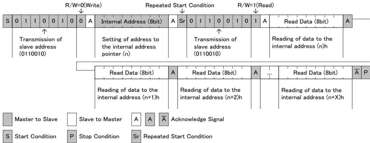
Fig. 10-5 I<sup>2</sup>C-Bus Data Transmission Read Format
