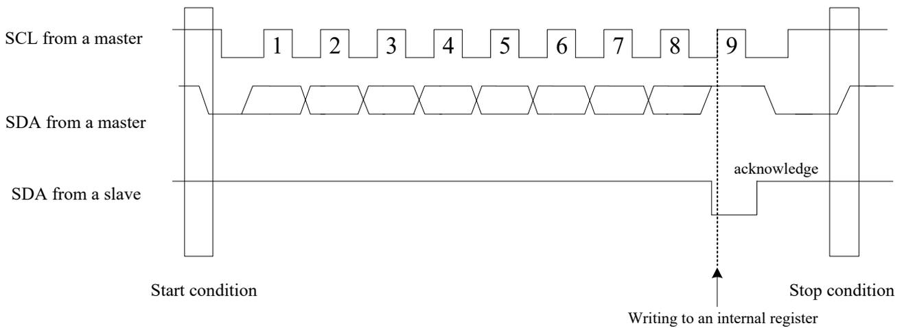
Fig. 10-3 I<sup>2</sup>C-Bus Internal Register Write-in Timing
