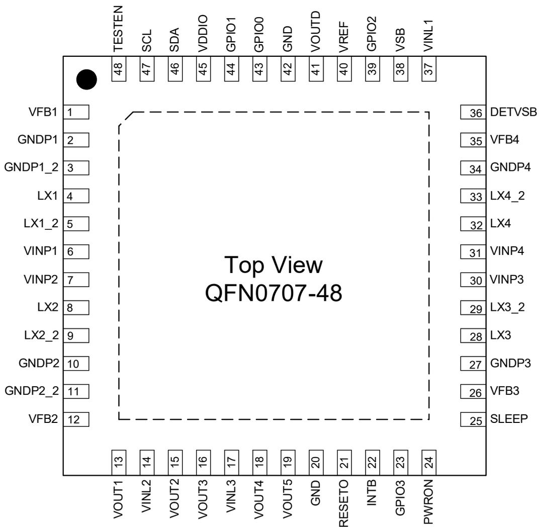
Fig. 5-1 Pin Configuration
