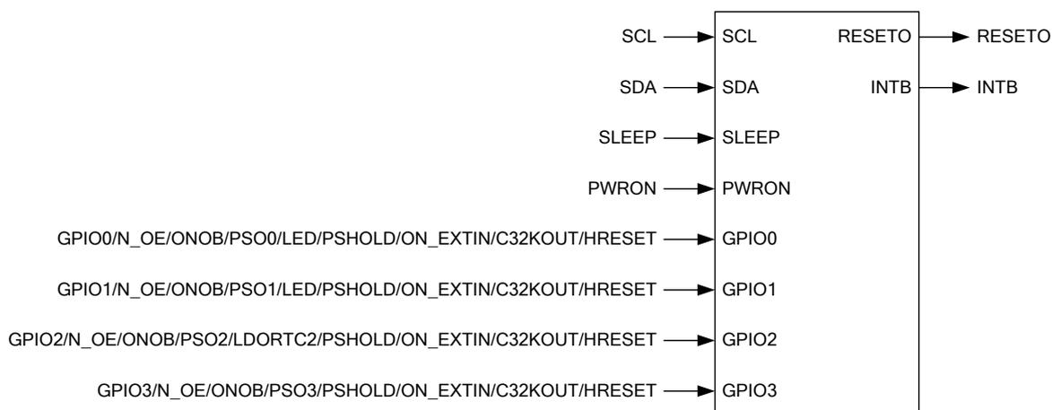
Fig. 8-1 The function of pins in Normal mode
