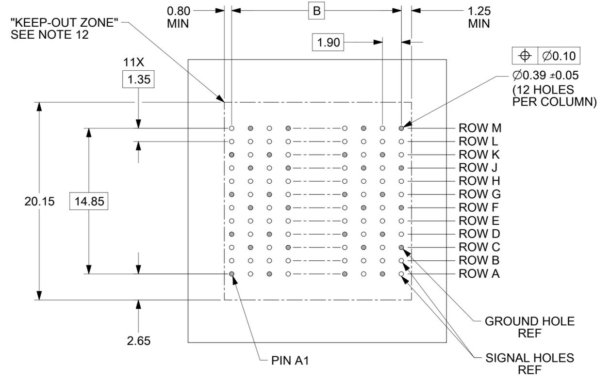
VERTICAL RECEPTACLE HOLE PATTERN (CONNECTOR SIDE)
