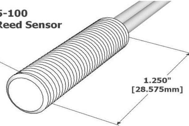
All measurements are in Inches [millimeters]
