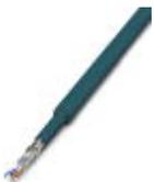
CAT5-SF/UTP cable (J-02YS(ST)C HP 2 x 2 x 24 AWG), heavy-duty installation cable, 2 x 2 x 0.22 mm<sup>2</sup>, solid conductor, shielded, outer sheath: 7.8 mm diameter, inner sheath: 5.75 mm ± 0.15 mm diameter
