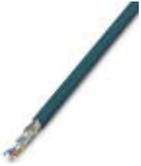
CAT5-SF/UTP cable (J-LI02YS(ST)C H 2 x 2 x 26 AWG), light-duty, flexible installation cable 2 x 2 x 0.14 mm<sup>2</sup>, stranded, shielded, outer sheath: 5.75 mm ± 0.15 mm diameter
