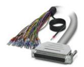
Assembled shielded round cable; connection 1: Single wires (37-position) (The wires are marked and fitted with ferrules. The braided shield is routed to a separate cable end.); connection 2: D-SUB socket strip (1x 37-position); cable length: 6 m
