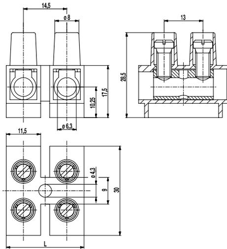
The socket terminal strip 327-FU with raised base and a pitch of 14,5 mm is available in 1 to 12 pole design.
